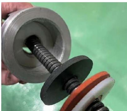
New stuffing box design
