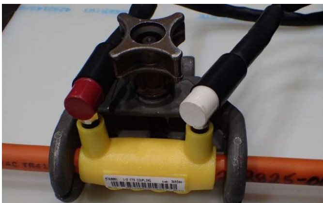
P/AC pipes being joined by a MDPE electrofusion coupling
