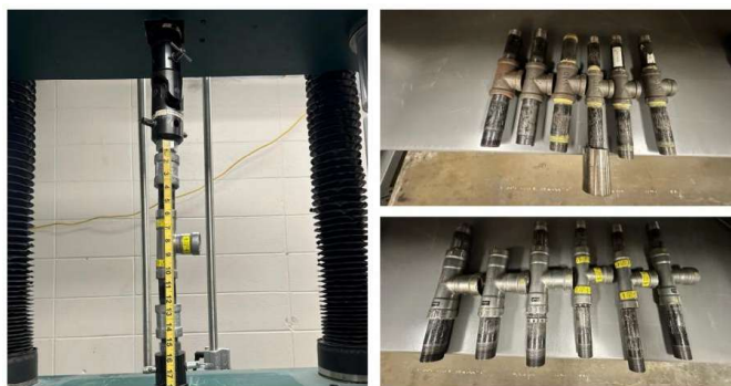
Tensile test being run and samples that were subjected to the test.
