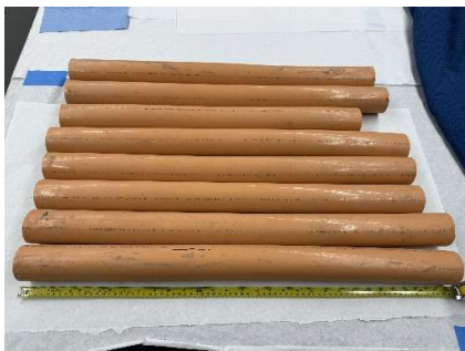
Aldyl A Pipe Samples; MDPE Pipe Samples; MDPE Pipe Samples – Dog bones
