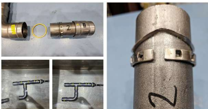
Burst test conducted in a 2-in Viega MegaPress G Manifold.
