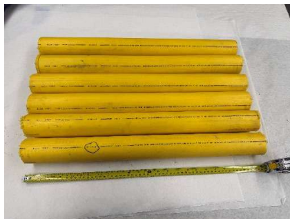
Aldyl A Pipe Samples; MDPE Pipe Samples; MDPE Pipe Samples – Dog bones
