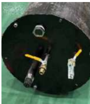
Downstream cap containing flowmeter and camera
