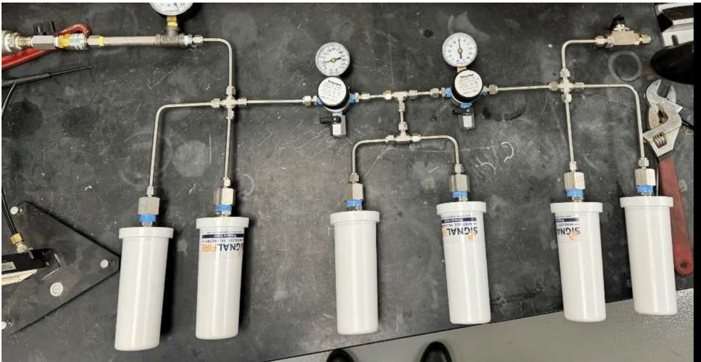
LoRaWAN-enabled Pressure Sensors Test Setup
