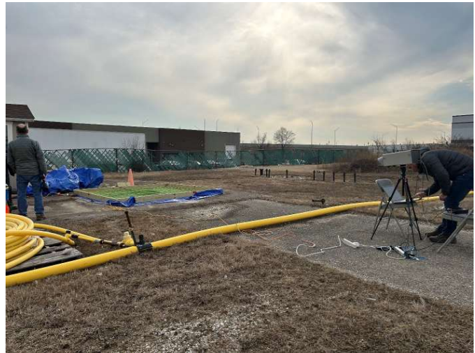
Outdoor testing using simulated underground leak.
