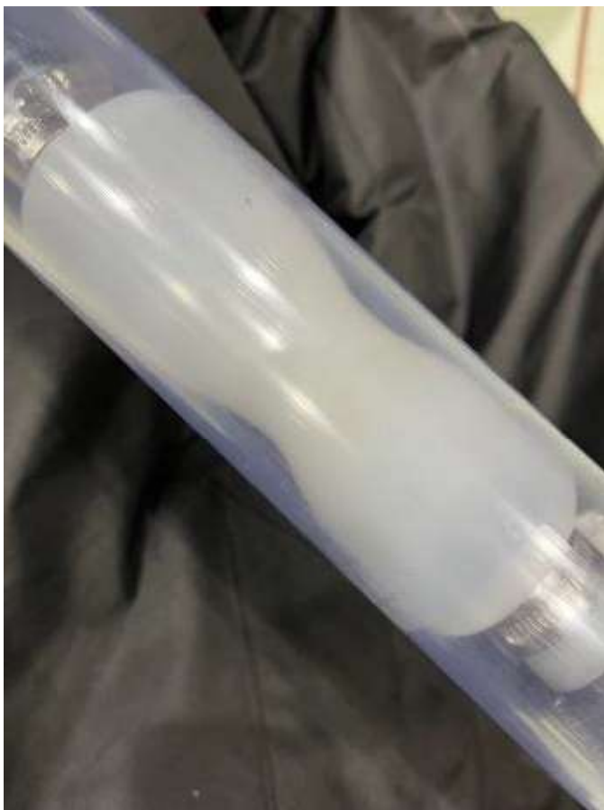
7-in Version of 2 IPS Balloon Stopper from OTD 5.22.n
