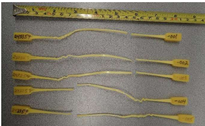
MDPE Tensile Specimens
