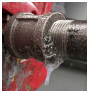
Leak detection size of bubbles prior to repair; right: example of repaired leak after putty is applied.
