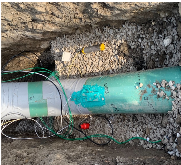
Sensors on pipe and in soil.
