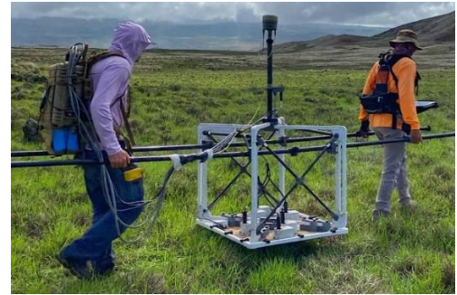
APEX operation in the chariot mode (top left) and hand-carry mode (middle) using the hand-carry attachment. The lightweight design (right) offers additional capabilities to survey in challenging environments.
