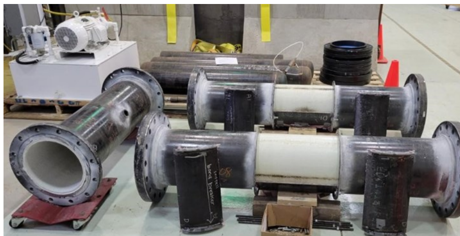
Preparation of the Repaired Pipe Sample for Internal Pressure Tests
