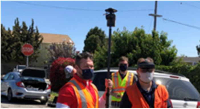
HoloLens 2 in use with Survey Pole with High- Accuracy GNSS Receiver
