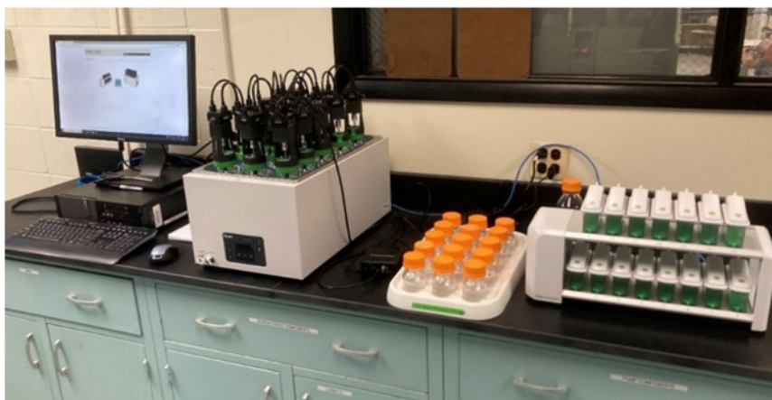
Components of BPC Gas Endeavor installed in GTI Energy's bioreactor room.
