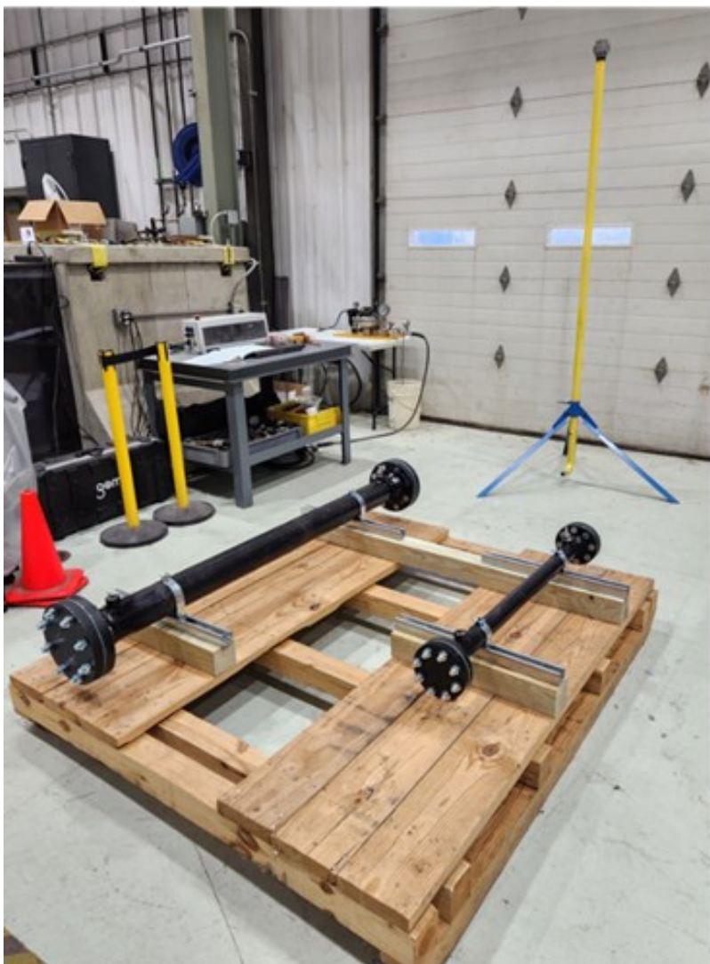
Figure 1 - Test Rig Pipes with vent flare stack, example H 2 Sensors, and example gas supply cylinders
