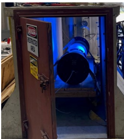
Preparation of the Repaired Pipe Sample for Internal Pressure Tests
