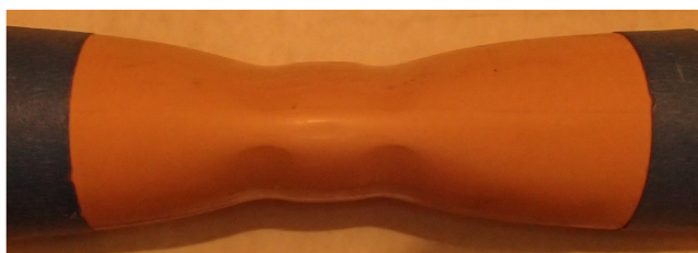
Specimen 222219-005 post squeeze at 0°C (32°F)
