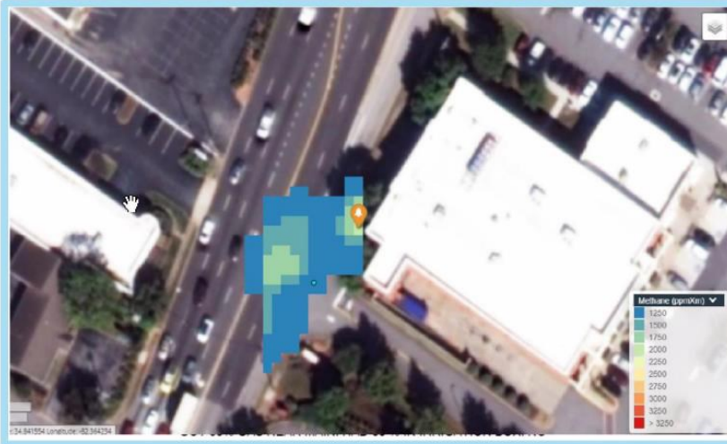
Measuring both plume and flow rates using Satelitytics' algorithms – source of leak marked with alert symbols chosen by customer
