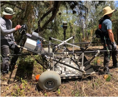
APEX operation in the chariot mode (top left) and hand-carry mode (middle) using the hand-carry attachment. The lightweight design (right) offers additional capabilities to survey in challenging environments.
