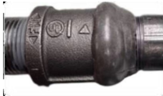
Leak detection size of bubbles prior to repair; right: example of repaired leak after putty is applied.
