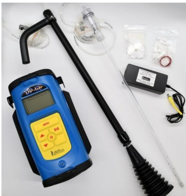
DP-IR, walking probe (black), bar hole probe (clear);
