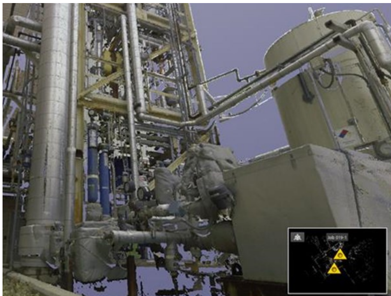
Leica scan with LiDAR point cloud and imagery combined
