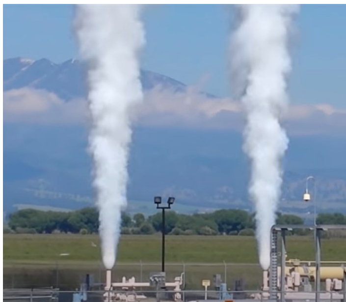
Figure 2: Gas venting to atmosphere during blow down operation
