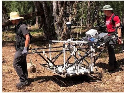
APEX operation in the chariot mode (top left) and hand-carry mode (middle) using the hand-carry attachment. The lightweight design (right) offers additional capabilities to survey in challenging environments.
