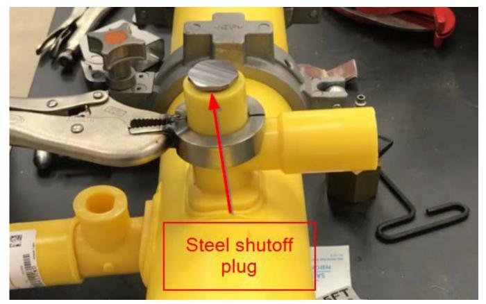
Main thread steel shutoff plug punched into the special threaded punch.
