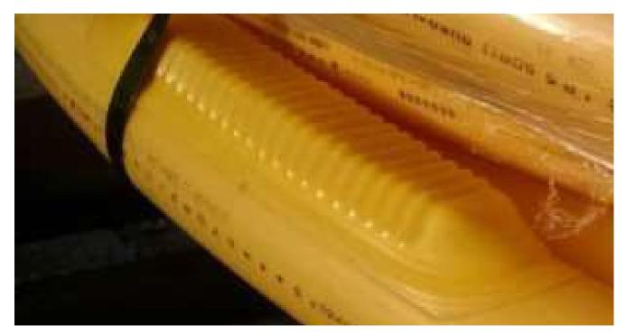
PE pipe with locatable tags attached.
