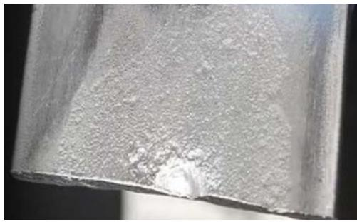
Mercury damage to aluminum.
