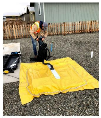
Measuring underground leak flow rate with a tarp enclosure and sampler.
