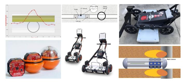
Researchers evaluated a variety of technologies to detect cross bores, including ground-penetrating radar, ultrasonic sensors, and acoustic-based technologies
