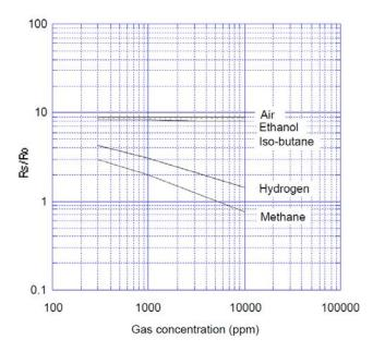
Methane and hydrogen response for a selected gas sensor
