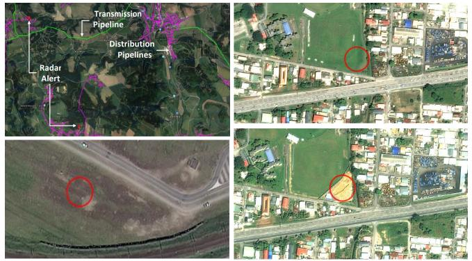
For locations where activity is detected that could potentially damage the pipeline, data from optical satellites is acquired. This enables the customer to analyze the location from the office.
