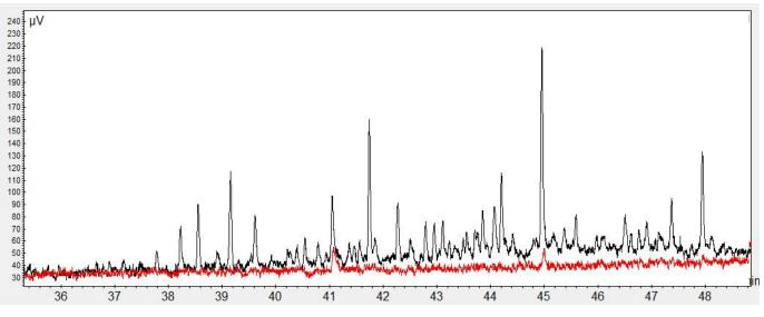
Gas chromatographic analysis of gases with and without (in red) odor masking.
