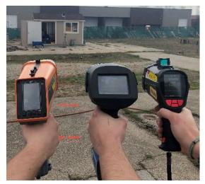
Evaluation of handheld laser methane detectors for an earlier project.
