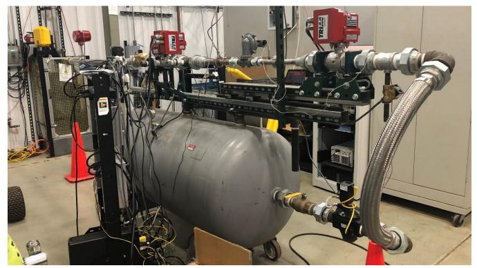
Regulator flow testing rig.
