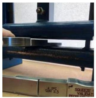
Utility personnel currently do not have tools to quickly check the performance of the squeeze tools. The use of a stop gap device as a calibration tool and/or validation tool before performing a squeeze on a PE pipe can lessen the risks associated with performing a squeeze improperly.
