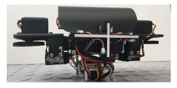
The tetherless PipeRider now enters its next phase of development – pitch control. Pitch control will give this pipe crawler two critical performance features: 1)the ability to stay aligned with a pipe's center axis regardless of the angle of the pipe underground and 2) the ability to turn a corner when an elbow or tee is encountered. PipeRider would roll to a vertical orientation for a turn in the horizontal plane.
