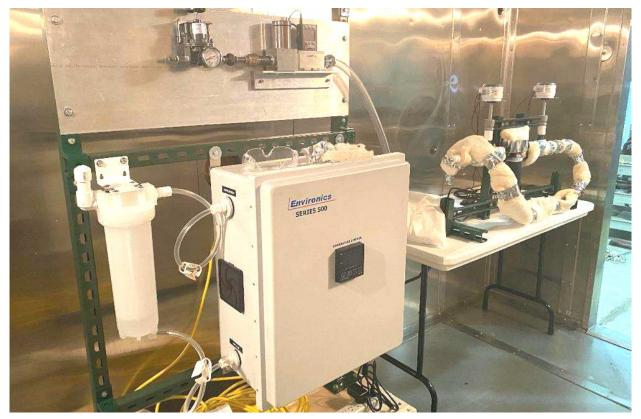
Water-vapor removal test rig.
