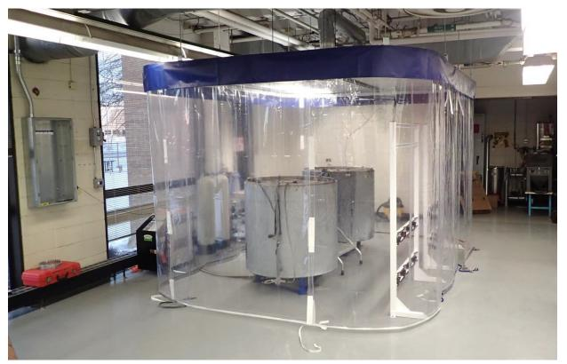
The enclosing test, water tanks, gas cylinder racks, water heaters, water-conditioning system, and ventilation duct are all in place. The tent enclosure confines any gas release and ensures the gas will be quickly extracted through the vent duct at the ceiling of the enclosure. with methane and methane/hydrogen blend. This task also includes a visual examination to count any existing SCG (slow crack growth) cracks.
