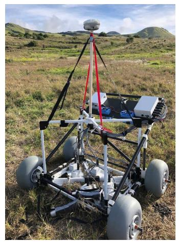
APEX is an advanced system for characterizing buried metal objects.
