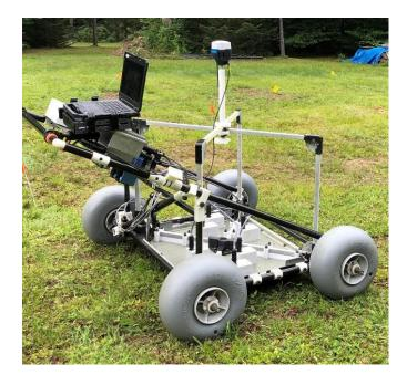
The solution is based on enhancing and adapting above-ground large-standoff 3D EM detection technology and supplementing the technology with an in-pipe mechanism to focus on congested areas and plastic materials. The combined solution will address most of the in-field conditions, including varying pipeline material, depth, and surface cover. The improved tools will provide access to the 3D data in near real time.
