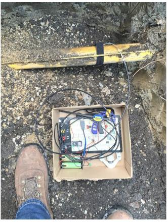
Field measurements on two-inch-diameter plastic main.
