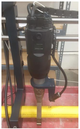
PE pipe repair machine heating tool assembly.
