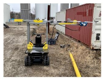
Fully constructed pushcart with the scanner attached.
