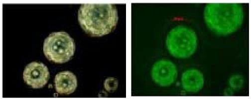
Smart corrosion-detector beads fluoresce a specific wavelength of light when in the presence of rust.
