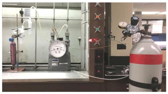
Setup to spike siloxane in methane gas.
