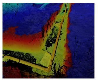
The goal of this project is to provide a digital twin for utilities to revisit underground work after backfill. This will improve field-crew safety (by alleviating the extra effort to enter the trench to collect data)
