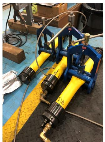
Pipe samples squeezed-off under pressure.
