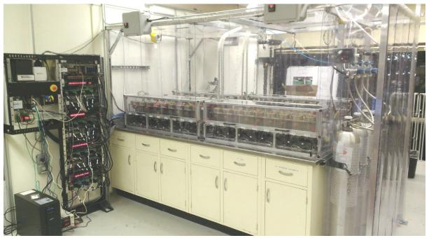
Rig for testing with flammable gases.
