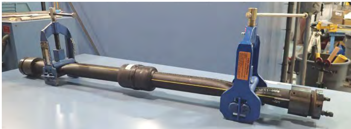
Sample with mechanical coupling, squeeze-off performed on both ends.
