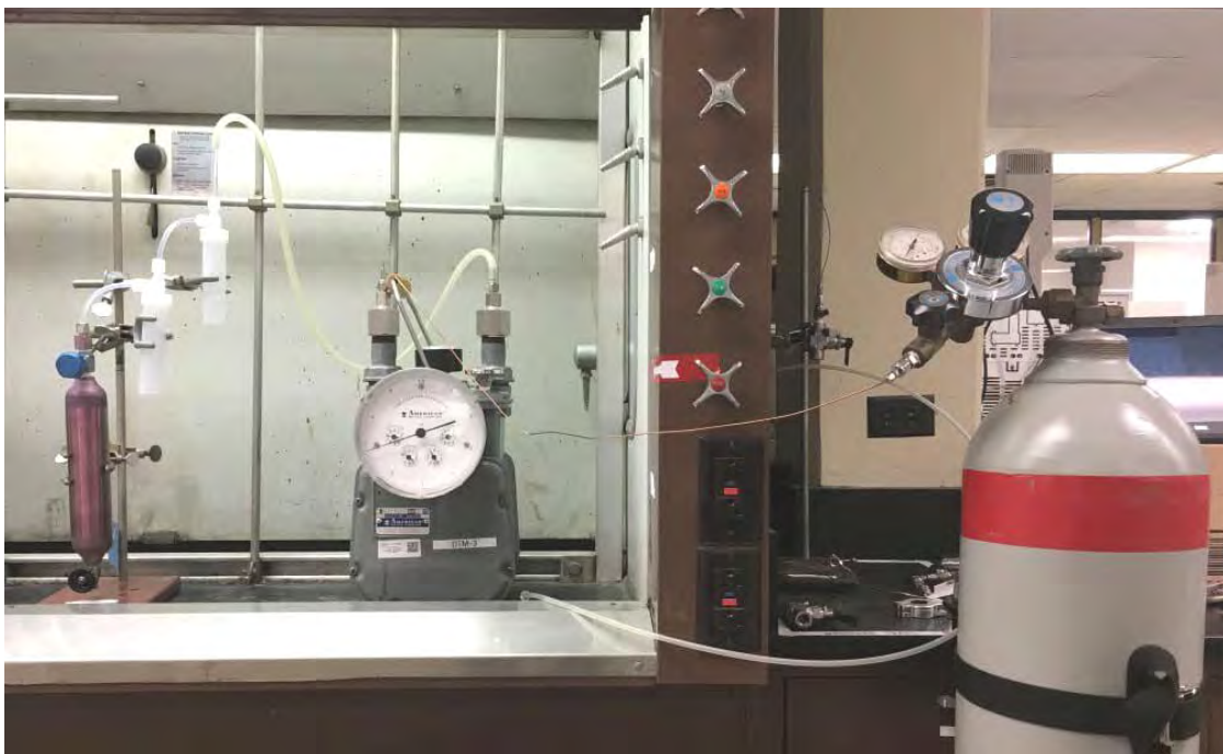
Setup to spike siloxane in methane gas.
