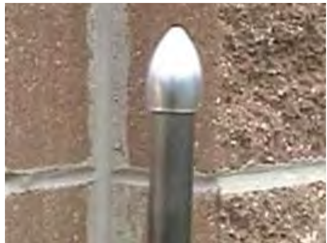
Prototype barhole tool with removable tip.
