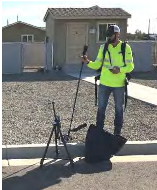
Measuring above-ground concentrations prior to barholing.
