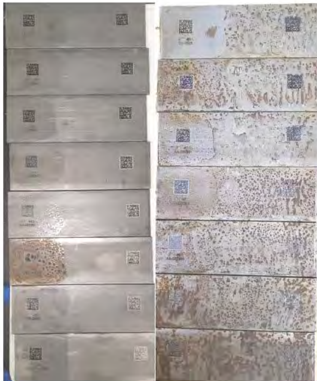
Salt-spray test of resins.
