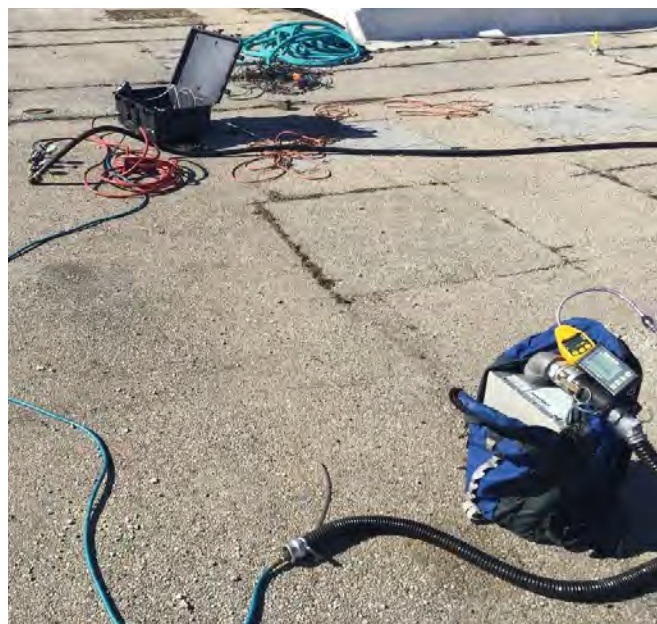
Measurements being made with the Hi-Flow™ sampler.
