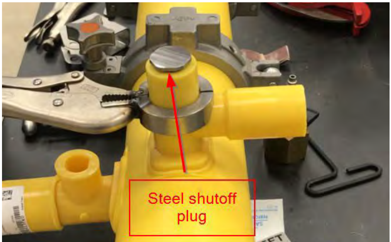
Main thread steel shutoff plug punched into the special threaded punch.
