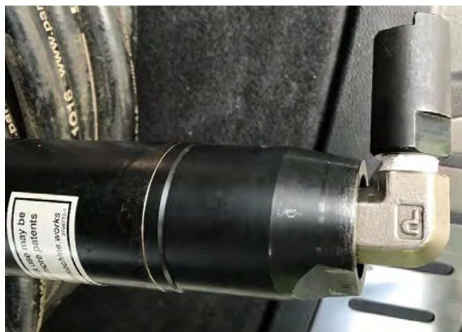
90-degree adapter on rear of piercing system.
