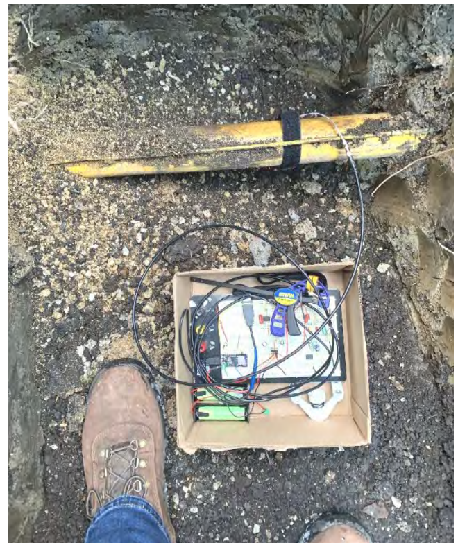
Field measurements on two-inch-diameter, plastic main.
