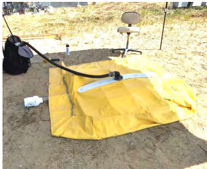
Enclosure used to determine the leak rate to validate the new methodology.
