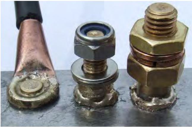
Examples of pin-brazed studs and stud-mount vibration sensor.
