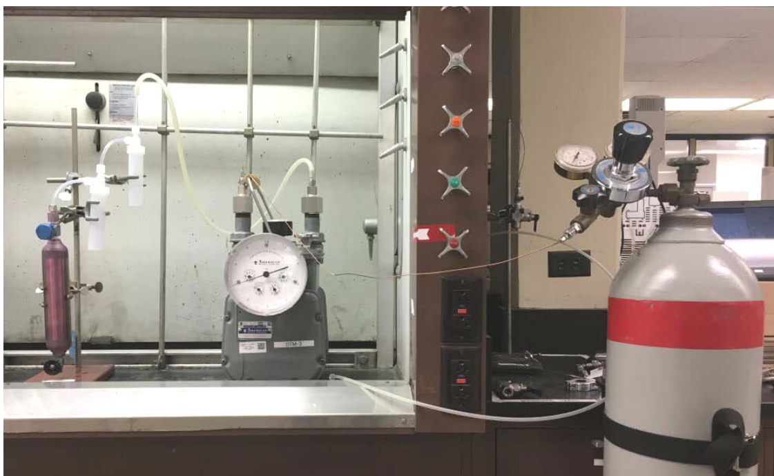
Setup to spike siloxane in methane gas.
