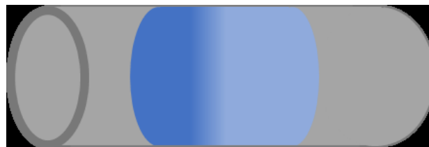
Figure 3. Example of mixing from excessive turbulent flow
