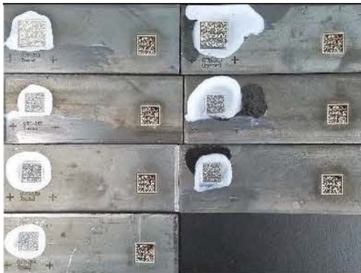
(Left) Laser-etched barcode samples before testing; (right) after corrosion testing.
