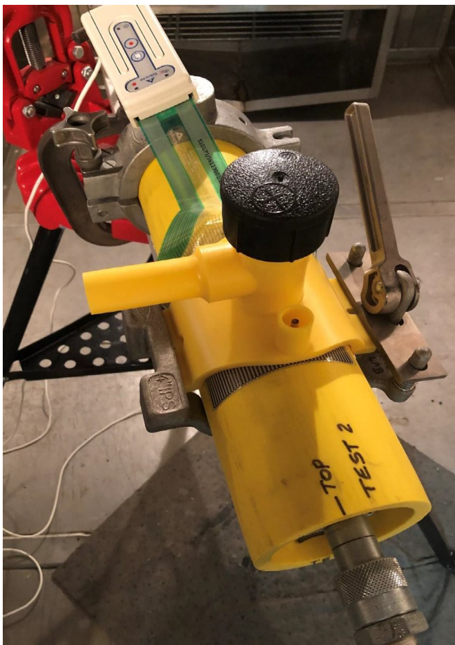
Pressure sensor used for pipe ovality check.
