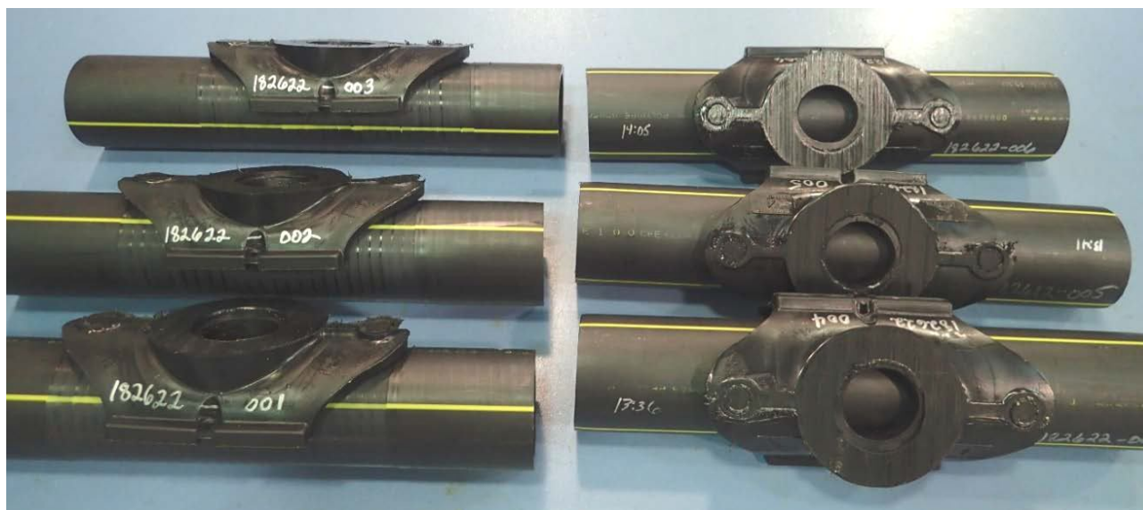
Scraped pipe samples on the left and non-scraped samples on the right.
