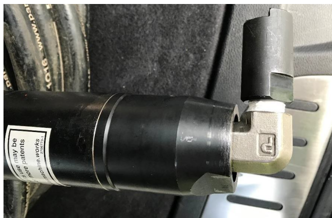
90-degree adapter on rear of piercing system.
