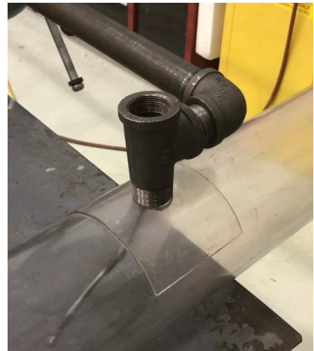
Left: Hinged stuffing box closed onto a two-inch pipe and cable behind a 20-inch bag. Right: Bag navigation and inflation testing.
