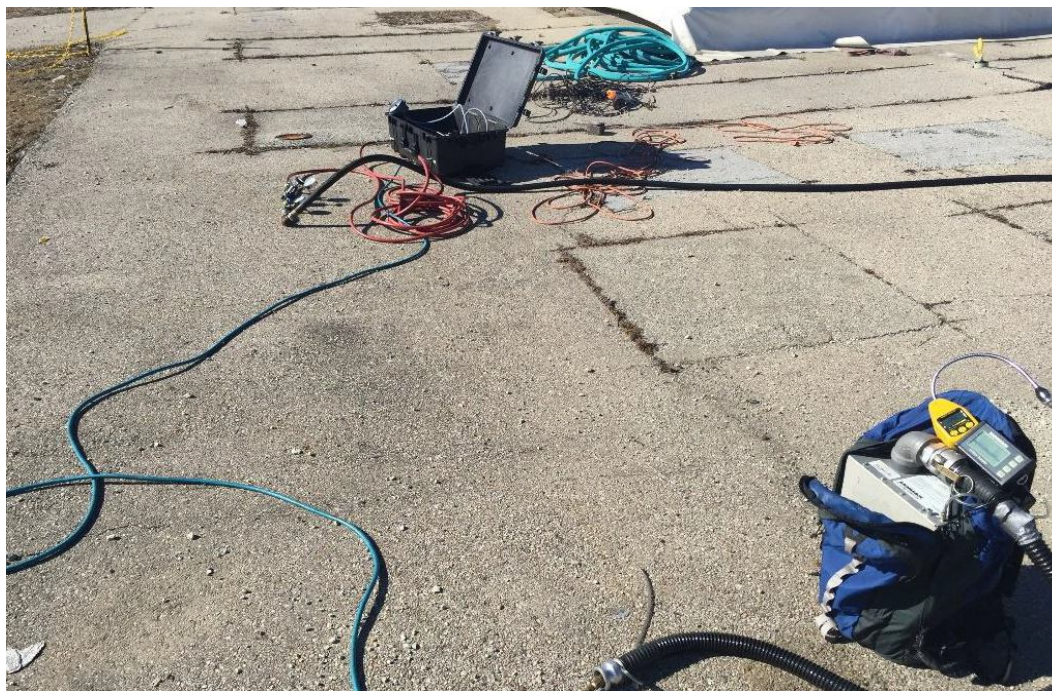
Measurements being made with the Hi-Flow™ sampler.
