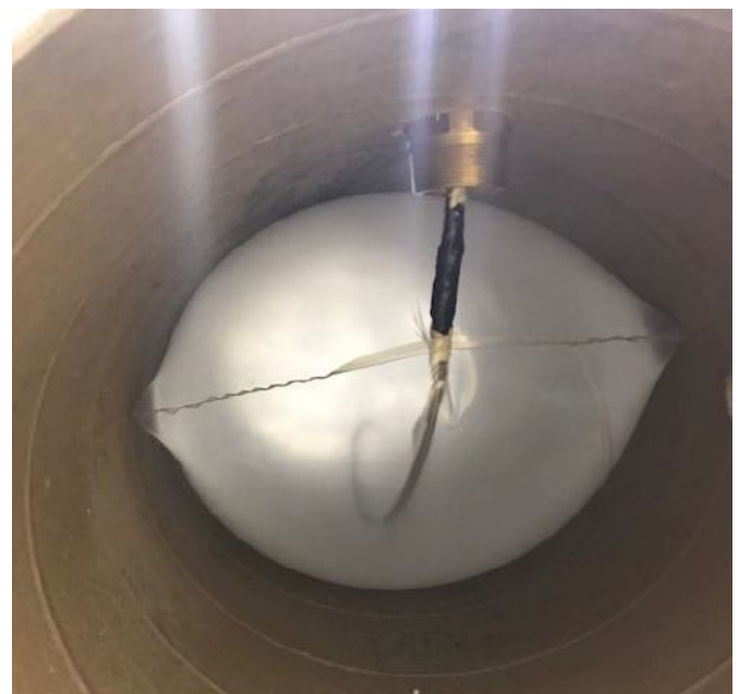
20-inch bag in 20-inch-diameter pipe.
