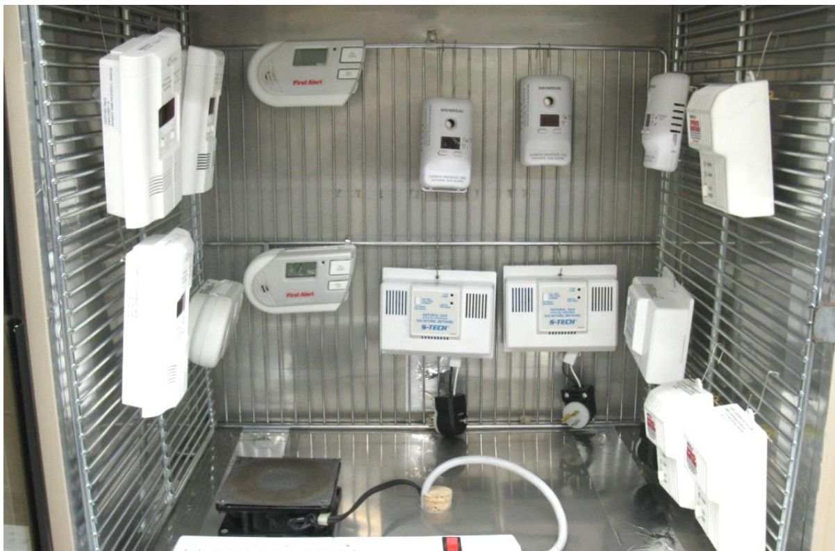
Methane detectors undergoing testing in an environmental test chamber.
