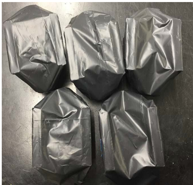
Conventional black-bag (not manufacturer packaging) before and after 350 hours of UV exposure.
