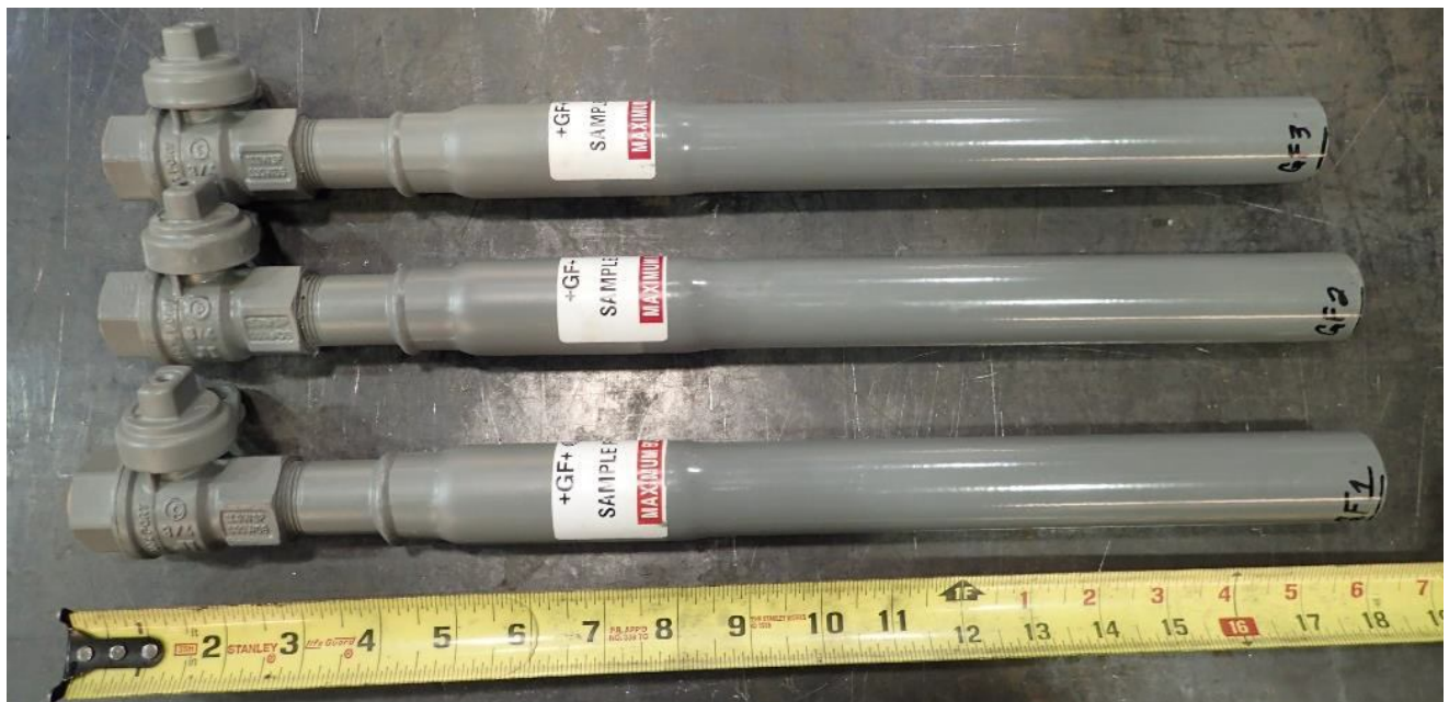
Anodeless service risers with pre-installed service valves cut to 18 inches.
