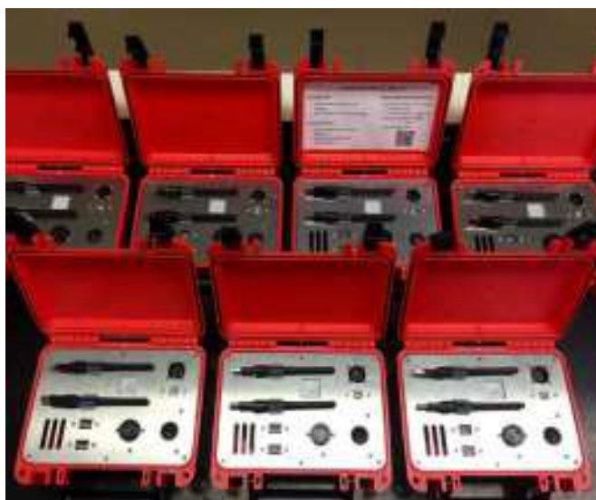
Networked methane sensors.
