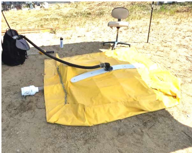
Enclosure used to determine the leak rate to validate the new methodology.
