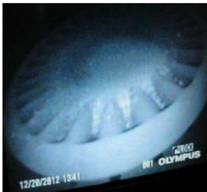
Silica deposits on water-heater burner.
