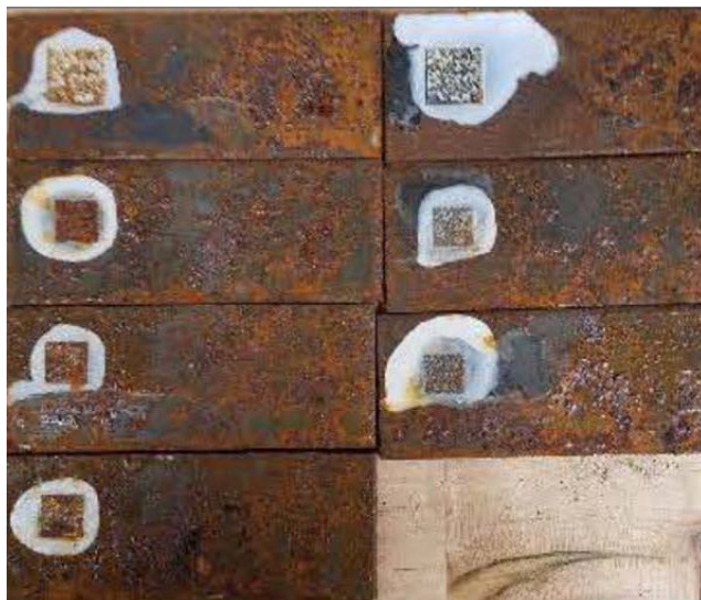
(Left) Laser-etched barcode samples before testing; (right) after corrosion testing.
