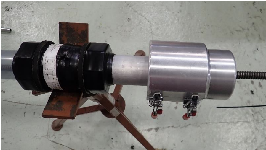
Left: Hinged stuffing box closed onto a two-inch pipe and cable behind a 20-inch bag. Right: Bag navigation and inflation testing.
