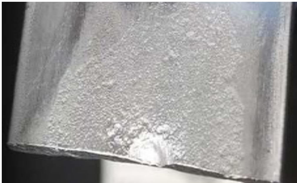
Mercury damage to aluminum.
