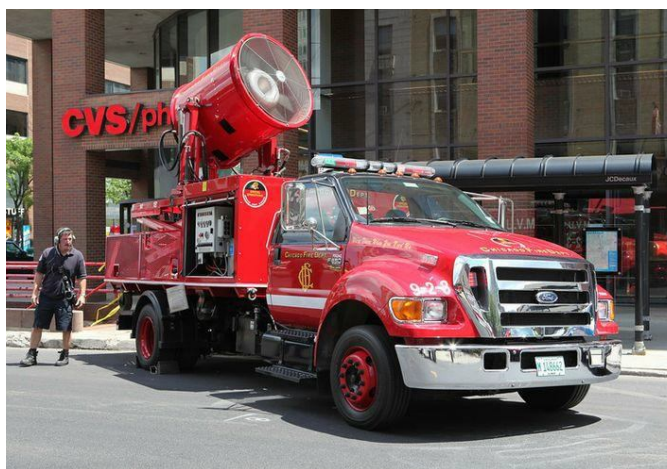
Positive-pressure mobile vehicle.
