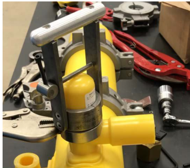
Cap being installed on service tee.
