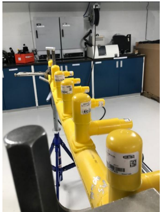
Twelve service-tee assemblies were built and tested.
