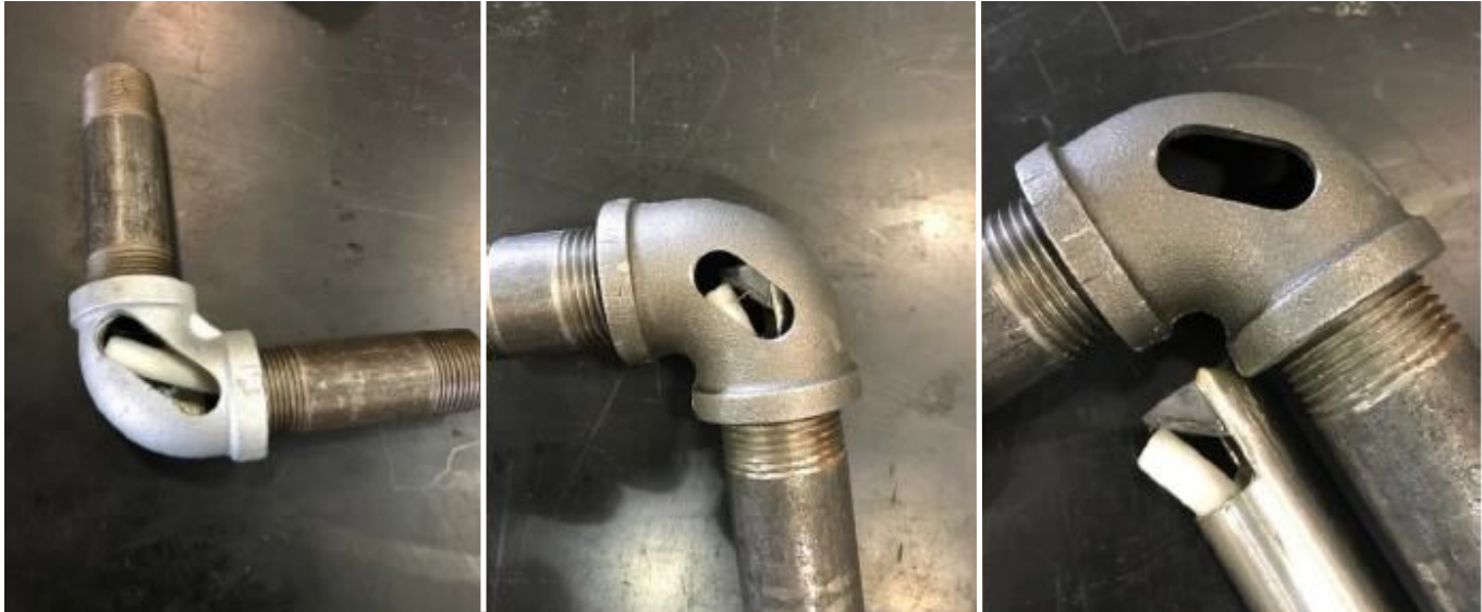
Modified electronic flow valve shell expanded inside pipe.
