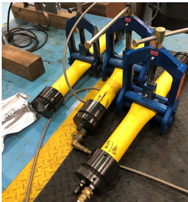
Pipe samples squeezed-off under pressure.
