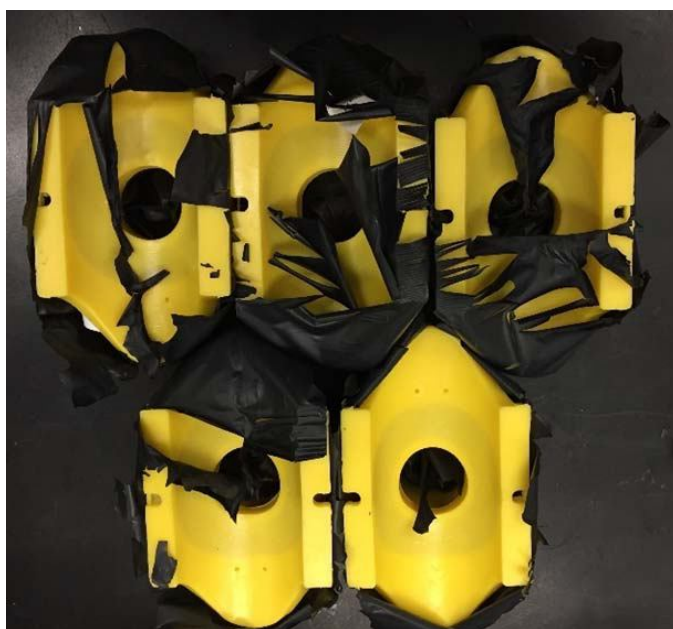
Conventional black-bag (not manufacturer packaging) before and after 350 hours of UV exposure.
