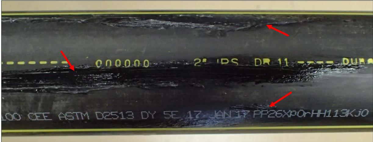
**Figure 18. Test Matrix 6 specimen after silicone grease contamination, red arrows point to the three lines**
