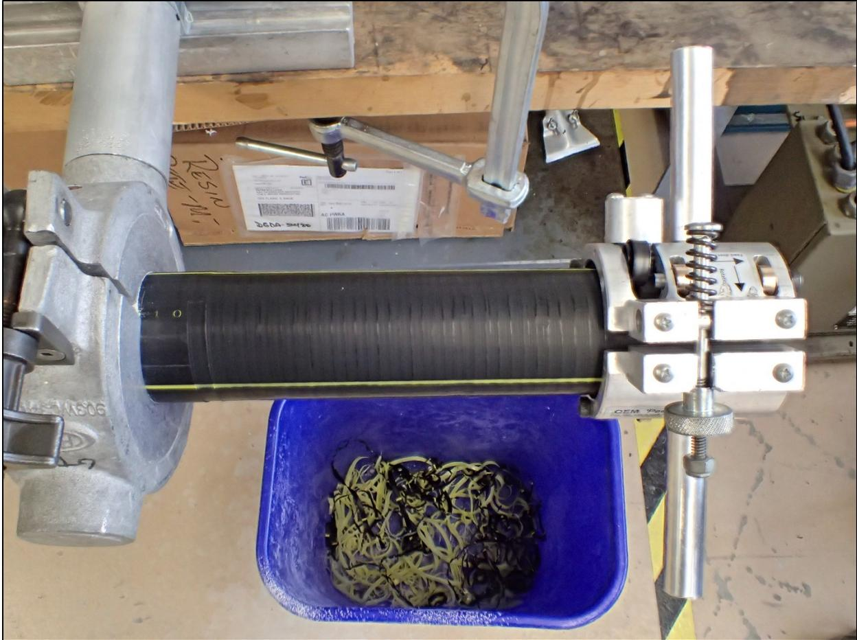
**Figure 165. Pipe contaminated with bentonite powder, end of scraping pass**
