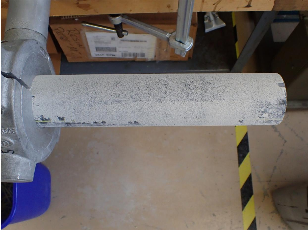
**Figure 161. Pipe contaminated with bentonite powder**
