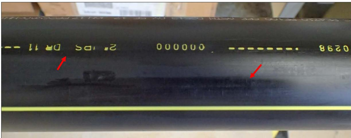
**Figure 20. Test Matrix 6 specimen after water wash and wipe. Red arrows show remaining silicone grease streaks.**
