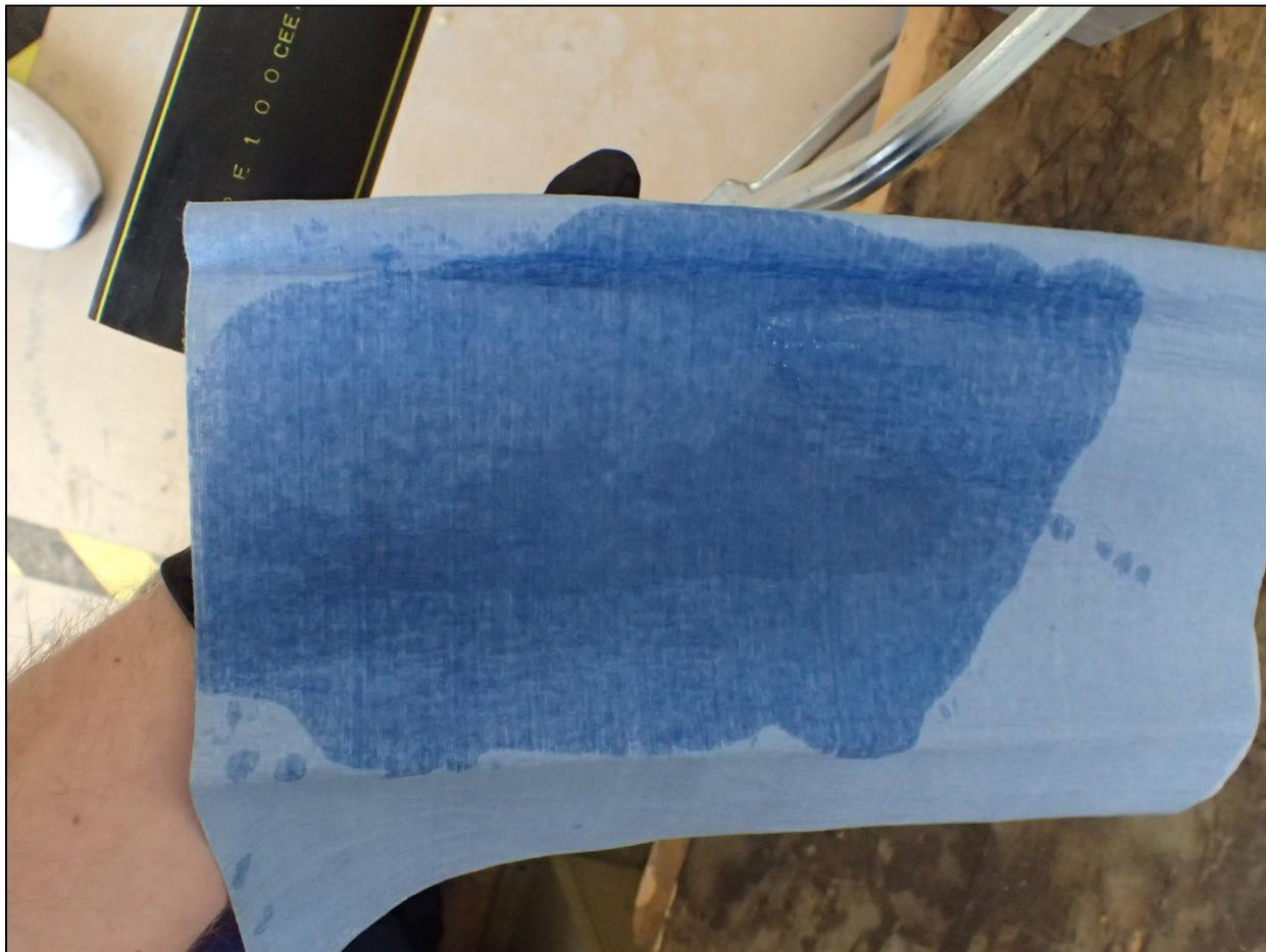
**Figure 159. Wetting of a lint-free wipe with a solvent**
