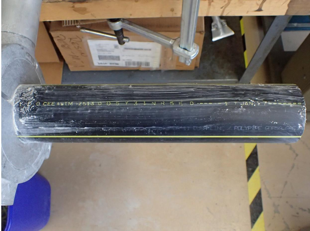
**Figure 162. Pipe contaminated with bentonite powder, after one solvent cleaning pass**
