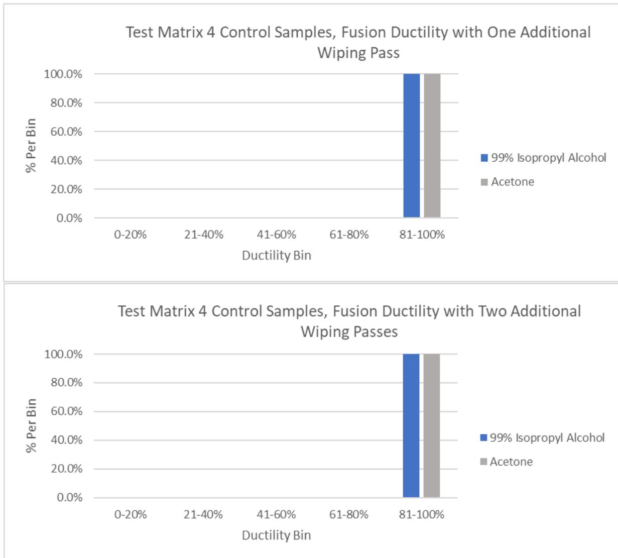
**Figure 13. Test Matrix 4 control sample (no contamination) results**
