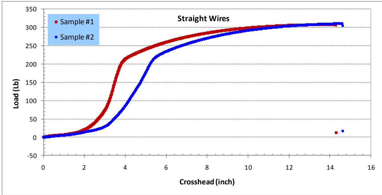
**Figure 36. Tensile Plots for Company B 10 AWG Soft Drawn Copper Wire\***
