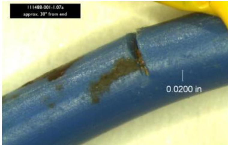
**Figure 17. Break of Insulation Jacket (#1) on Field Tested Company D-12 AWG Copper Clad Steel Wire**
