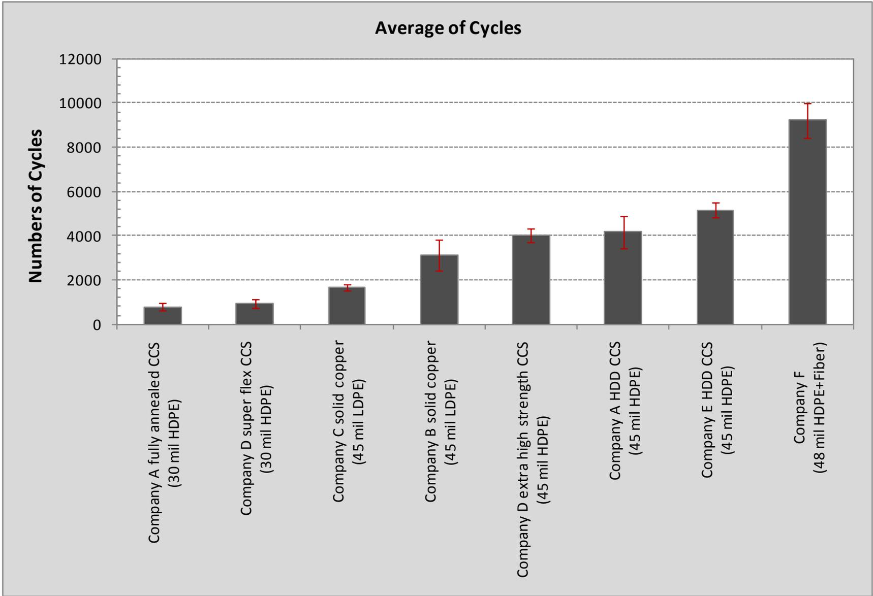
Figure 6. Scrape Test Results
