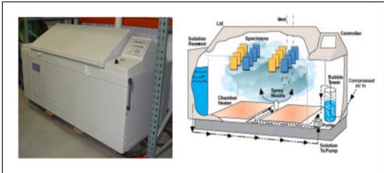
Figure 9. Cyclic Salt Fog Tester
