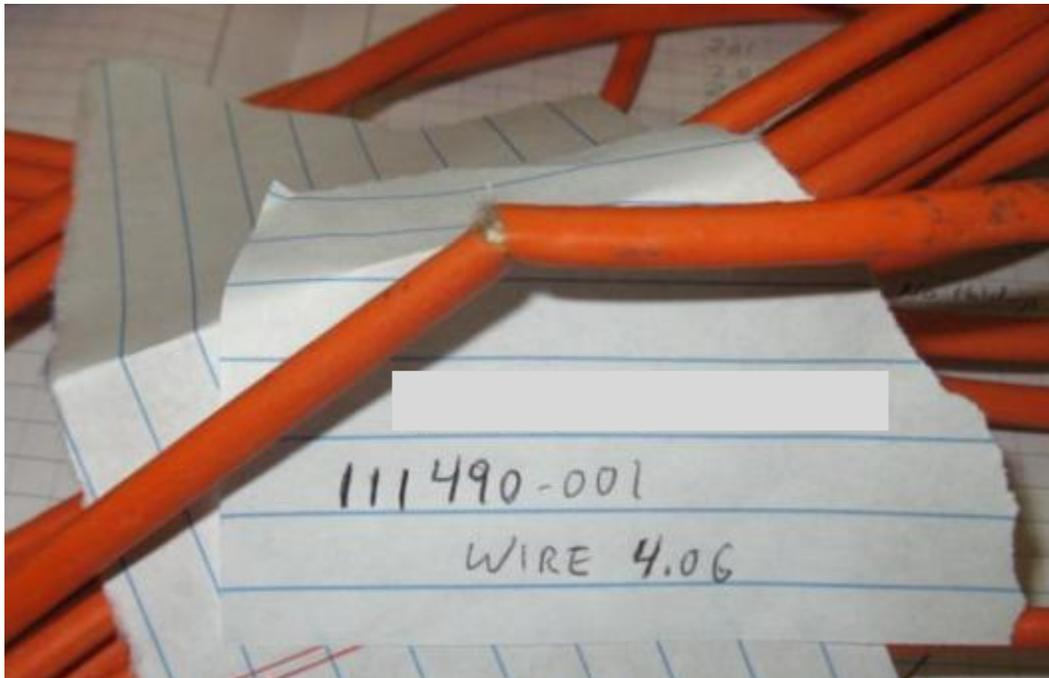
**Figure 12. Break of Insulation Jacket on Field Tested Company F Wire**
