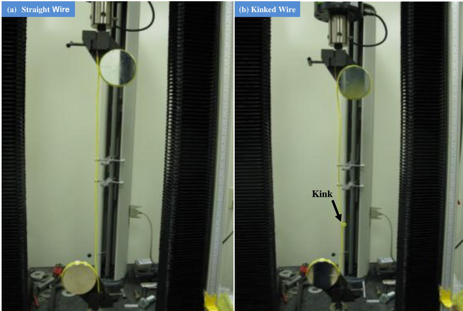
Figure 2. Wire Tensile Test Setup
