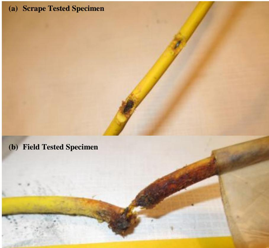
**Figure 10. The Corroded Company E-HDD-CCS Test Specimens after 2000 hr CCT-1 Test**
