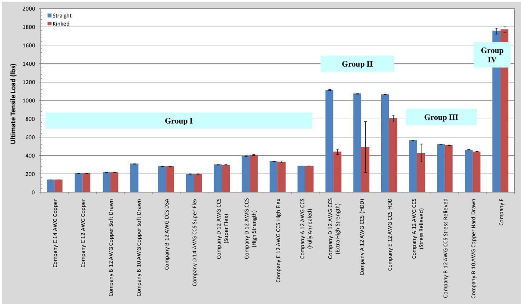
Figure 8. Ultimate Tensile Strength of the Straight and Kinked Tracer Wires
