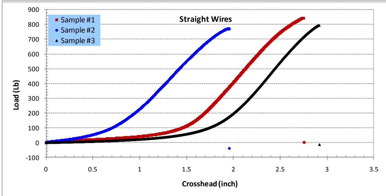
**Figure 29. Tensile Plots for Straight and Kinked Company E HDD 12 AWG Copper Clad Steel Wire**
