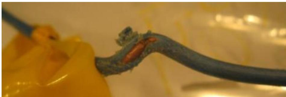
**Figure 19. Break of Insulation Jacket (#3) on Field Tested Company D-12 AWG Copper Clad Steel Wire**
