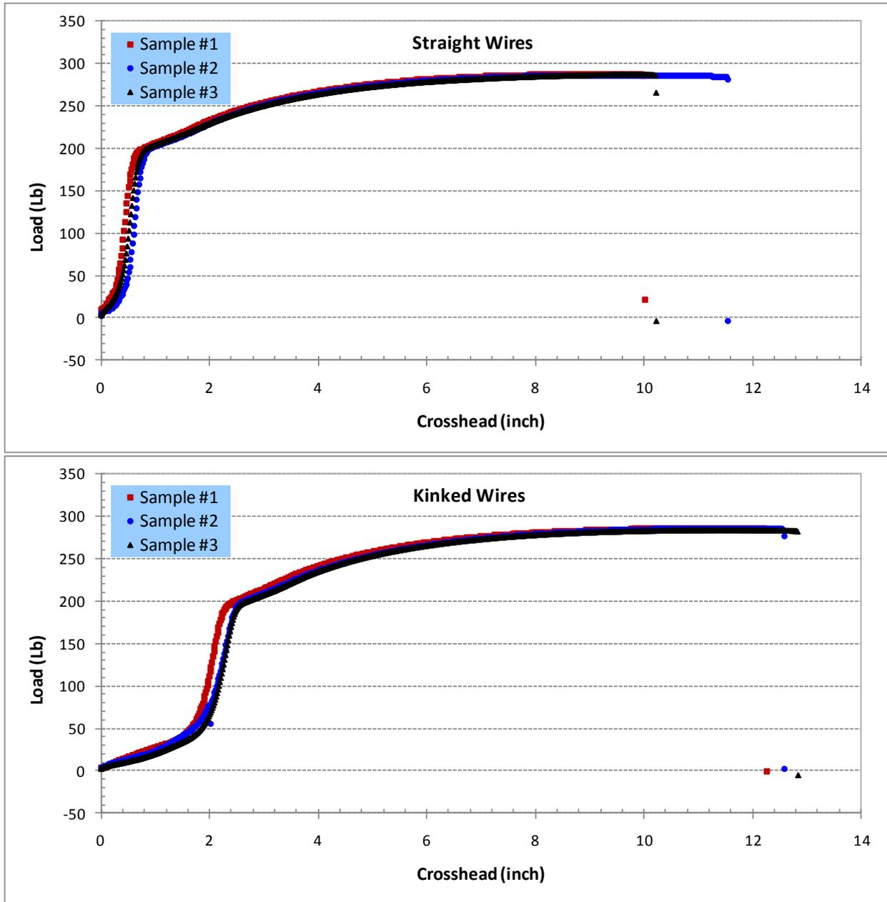
Figure 26. Tensile Plots for Straight and Kinked Company A 12 AWG Fully Annealed Copper Clad Steel Wire
