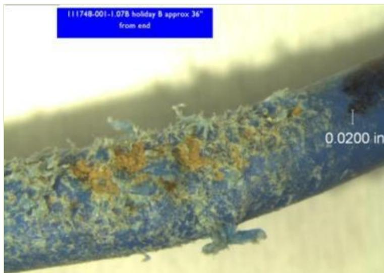
**Figure 18. Break of Insulation Jacket (#2) on Field Tested Company D-12 AWG Copper Clad Steel Wire**
