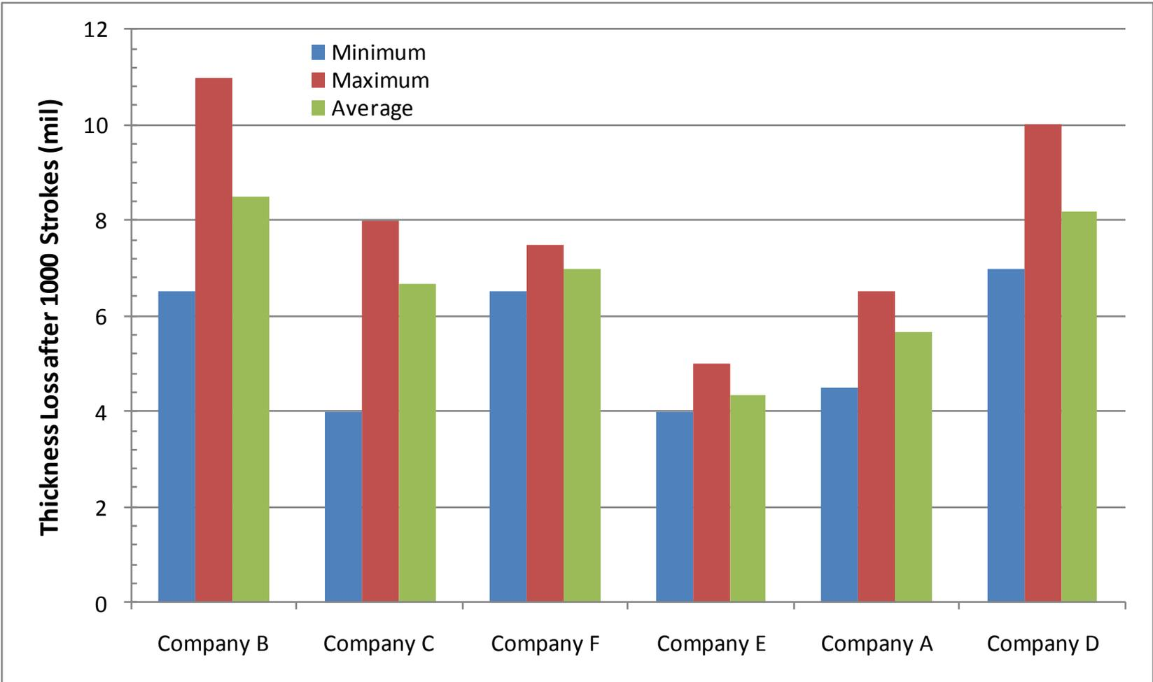
Figure 4. Taber Abrasion Test Results
