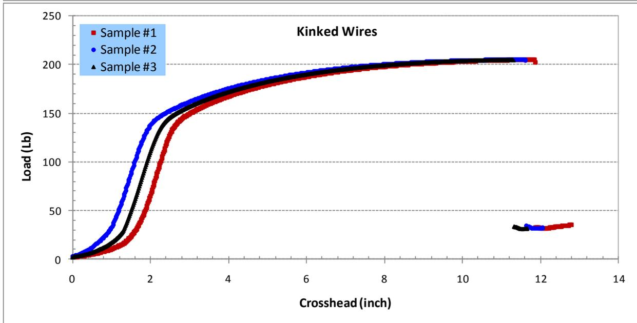
Figure 21. Tensile Plots for Straight and Kinked Company C 12 AWG Copper Wire
