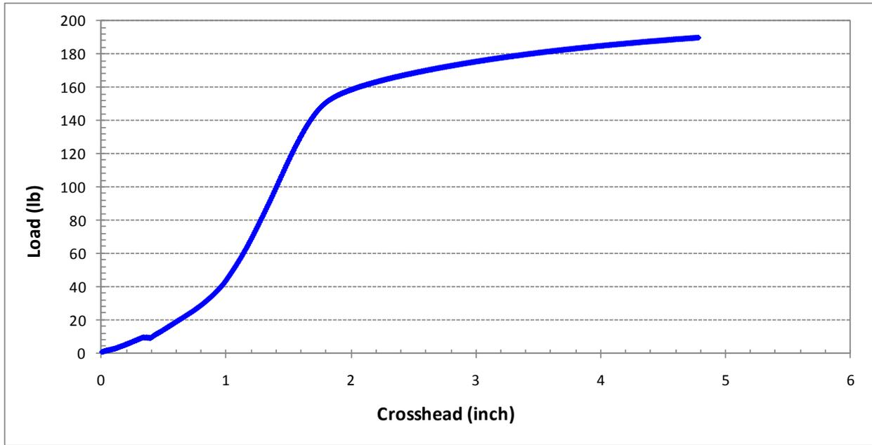
**Figure 39. Tensile Plot for Field Tested Company A 12 AWG Copper Clad Steel Wire (Holiday #2)**
