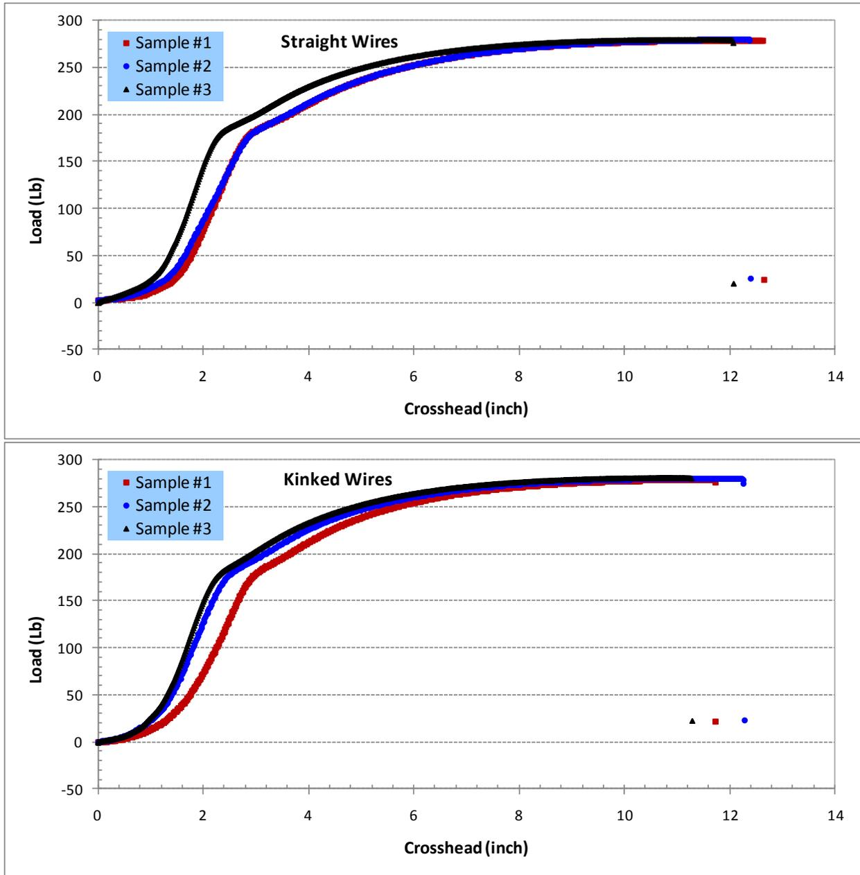
**Figure 33. Tensile Plots for Straight and Kinked Company B Dead Soft Annealed 12 AWG CCS Wire**
