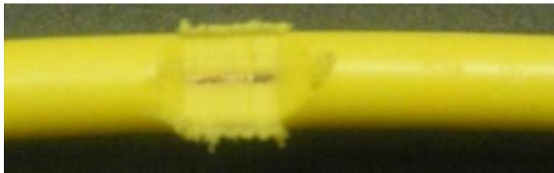
**Figure 5. Wire Sample after Scrape Test**
