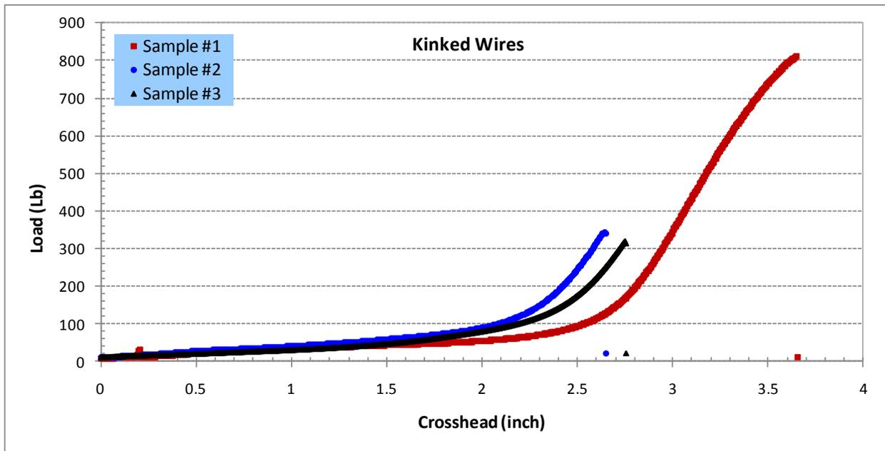
**Figure 28. Tensile Plots for Straight and Kinked Company A HDD 12 AWG Copper Clad Steel Wire**
