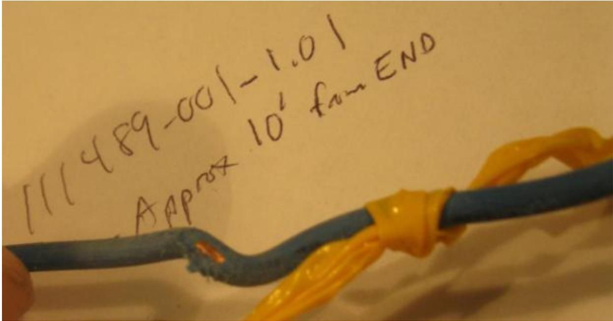
Figure 14. Break of Insulation Jacket (#2) on Field Tested Company A-12 AWG Solid Copper Wire
