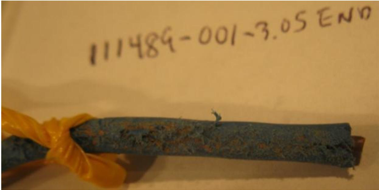
Figure 16. Break of Insulation Jacket (#4) on Field Tested Company A-12 AWG Solid Copper Wire
