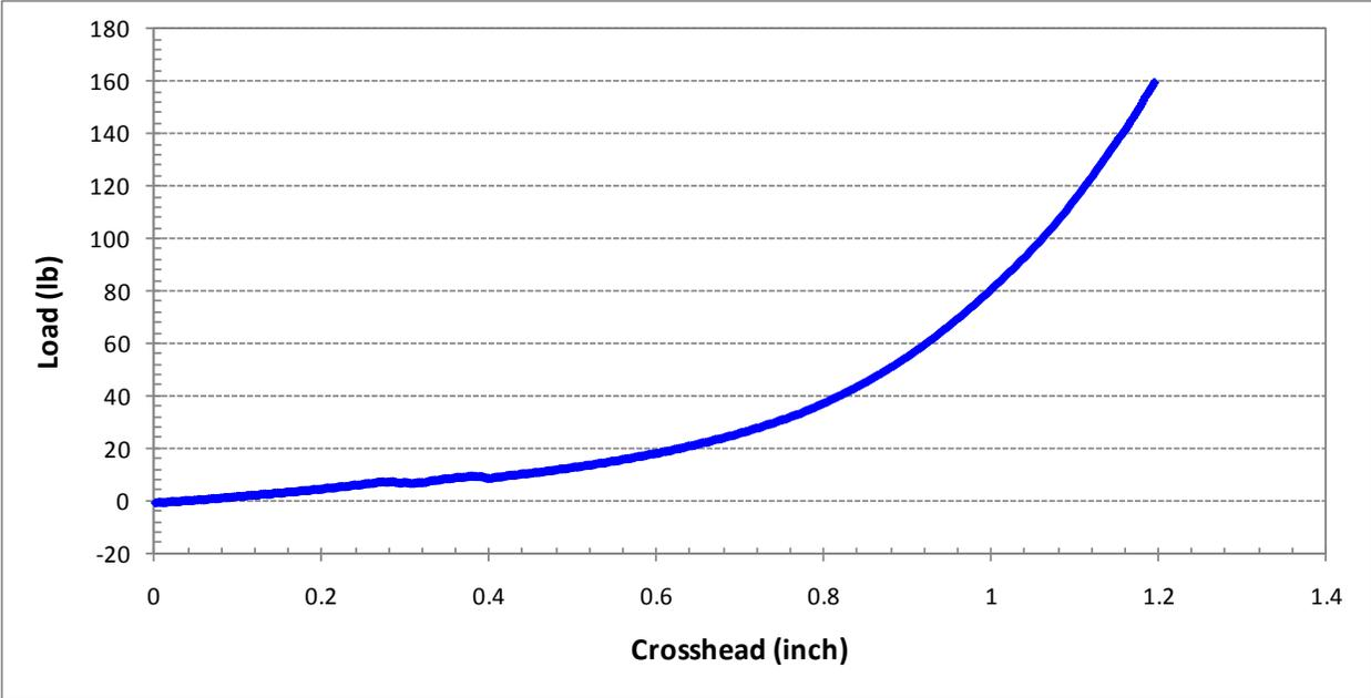
**Figure 37. Tensile Plot for Field Tested Company D 12 AWG Copper Clad Steel Wire**
