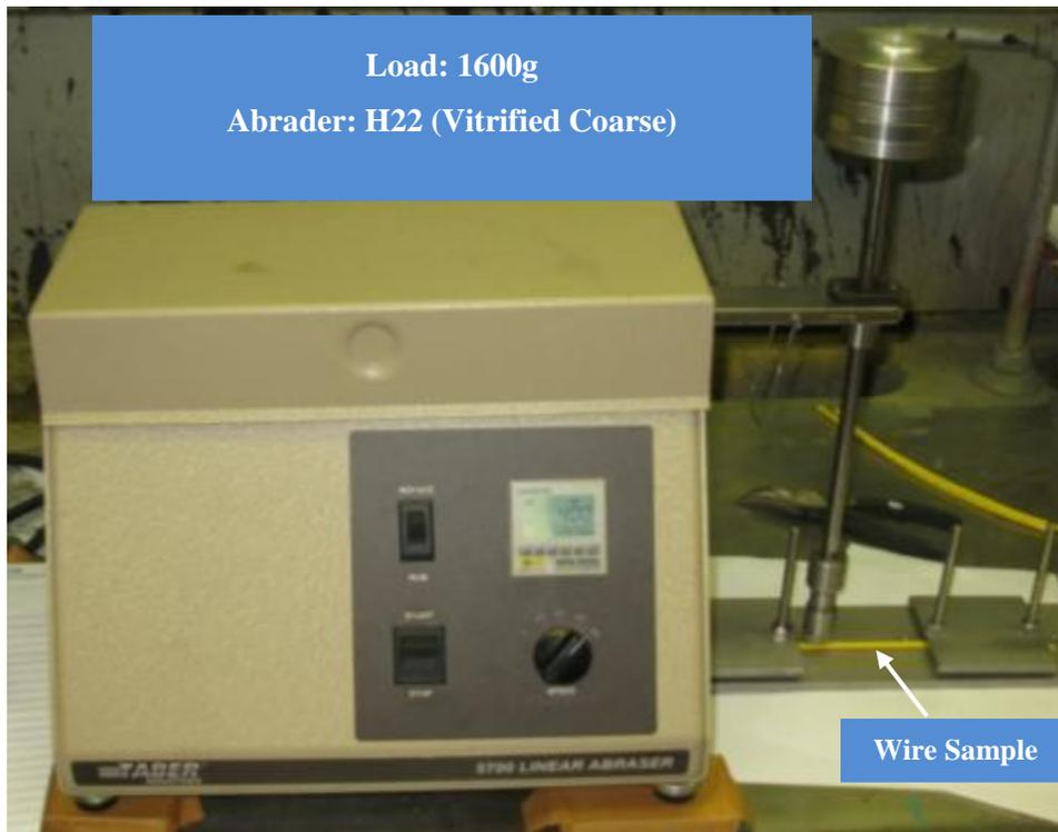
**Figure 3. Taber Abrasion Test Setup**
