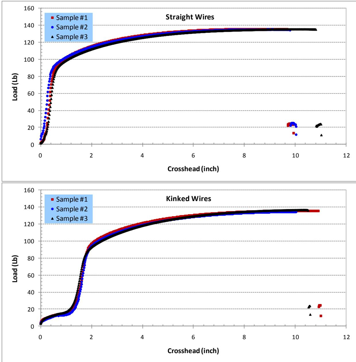
Figure 20. Tensile Plots for Straight and Kinked Company C 14 AWG Copper Wire
