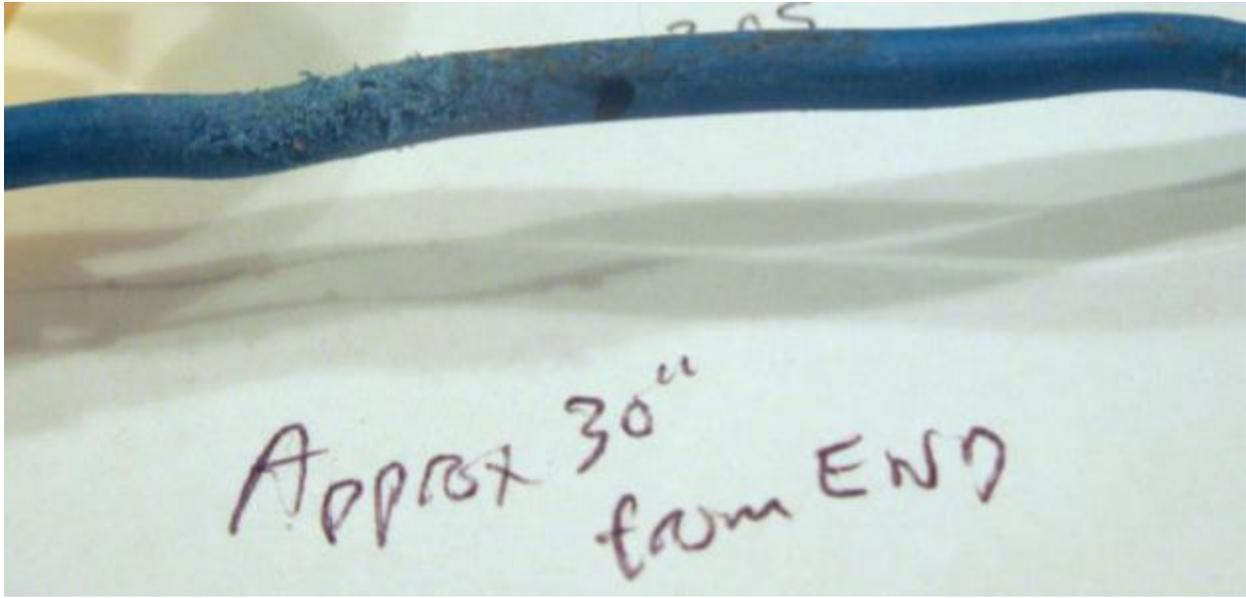
Figure 15. Break of Insulation Jacket (#3) on Field Tested Company A-12 AWG Solid Copper Wire
