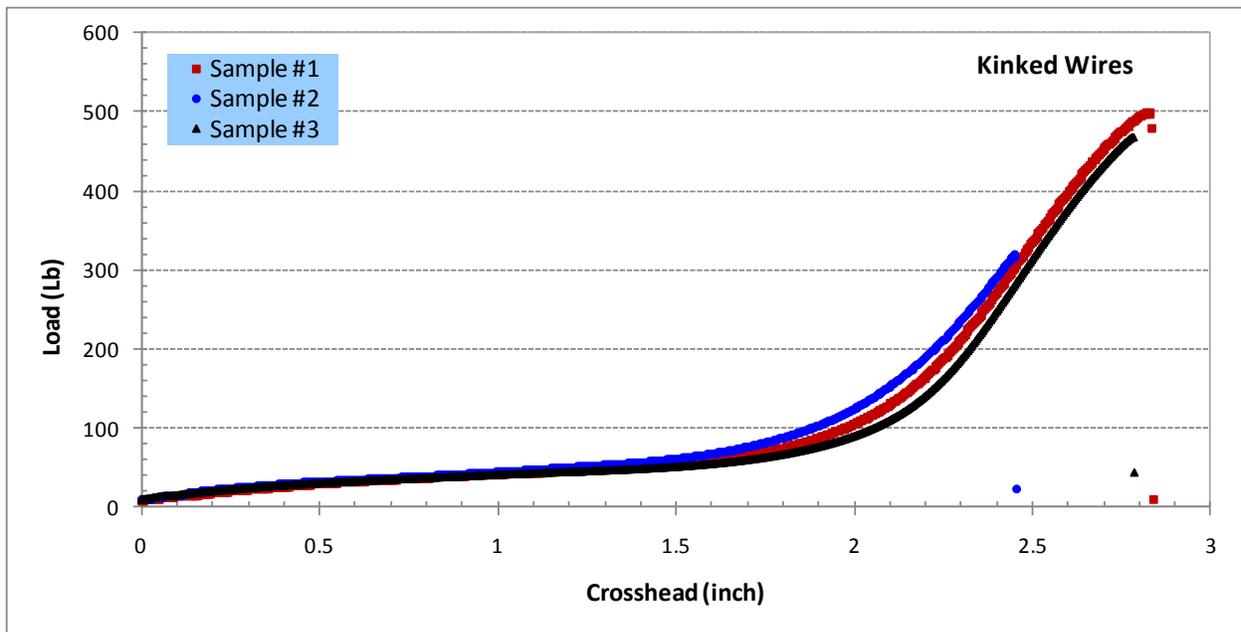
**Figure 27. Tensile Plots for Straight and Kinked Company A 12 AWG Stress Relieved Copper Clad Steel Wire**
