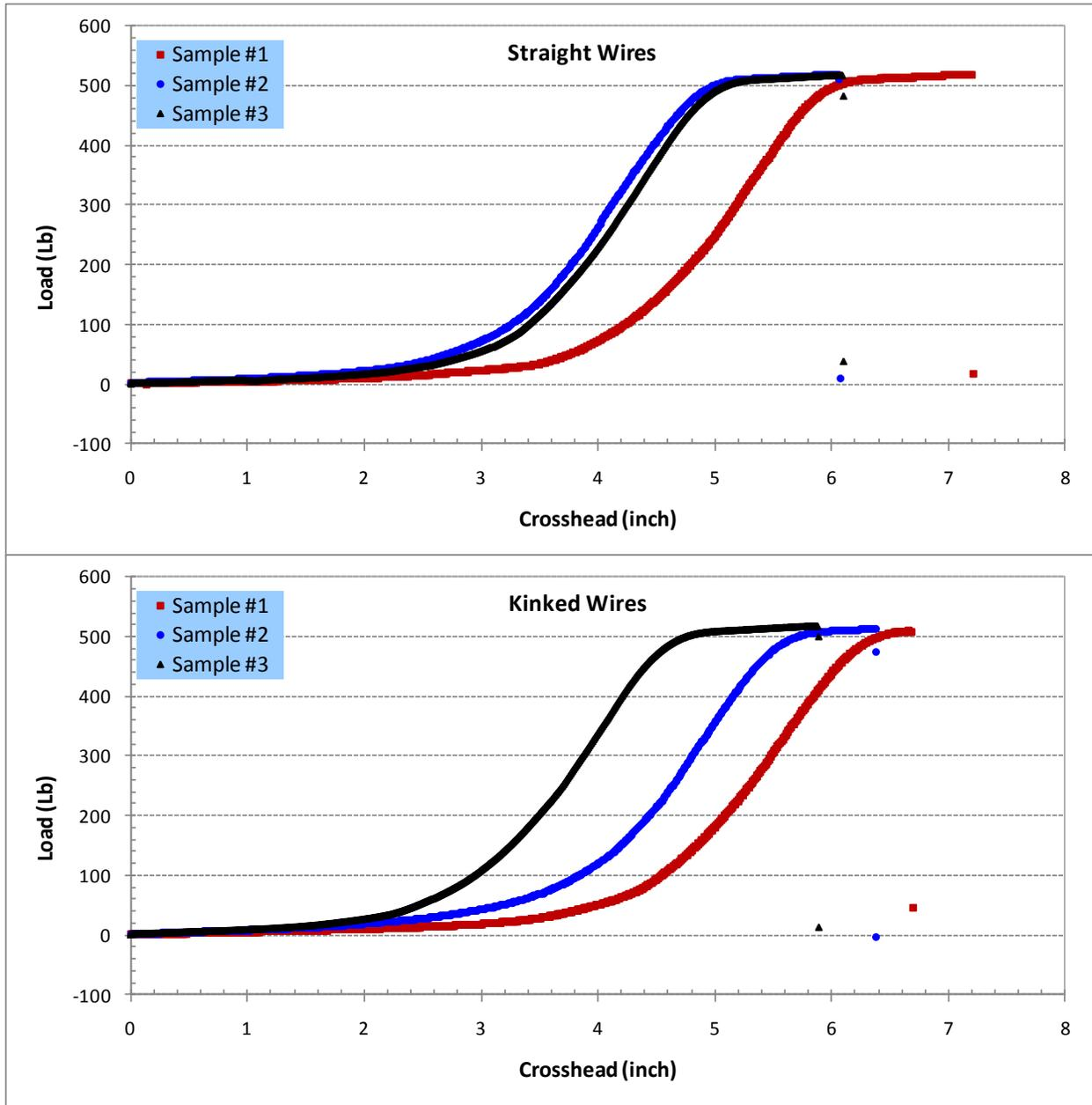
Figure 34. Tensile Plots for Straight and Kinked Company B Stress Relieved 12 AWG CCS Wire
