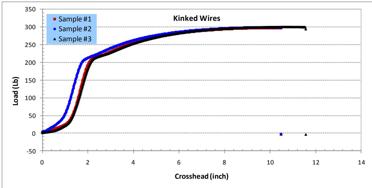
**Figure 24. Tensile Plots for Straight and Kinked Company D 12 AWG Super Flex Copper Clad Steel Wire**
