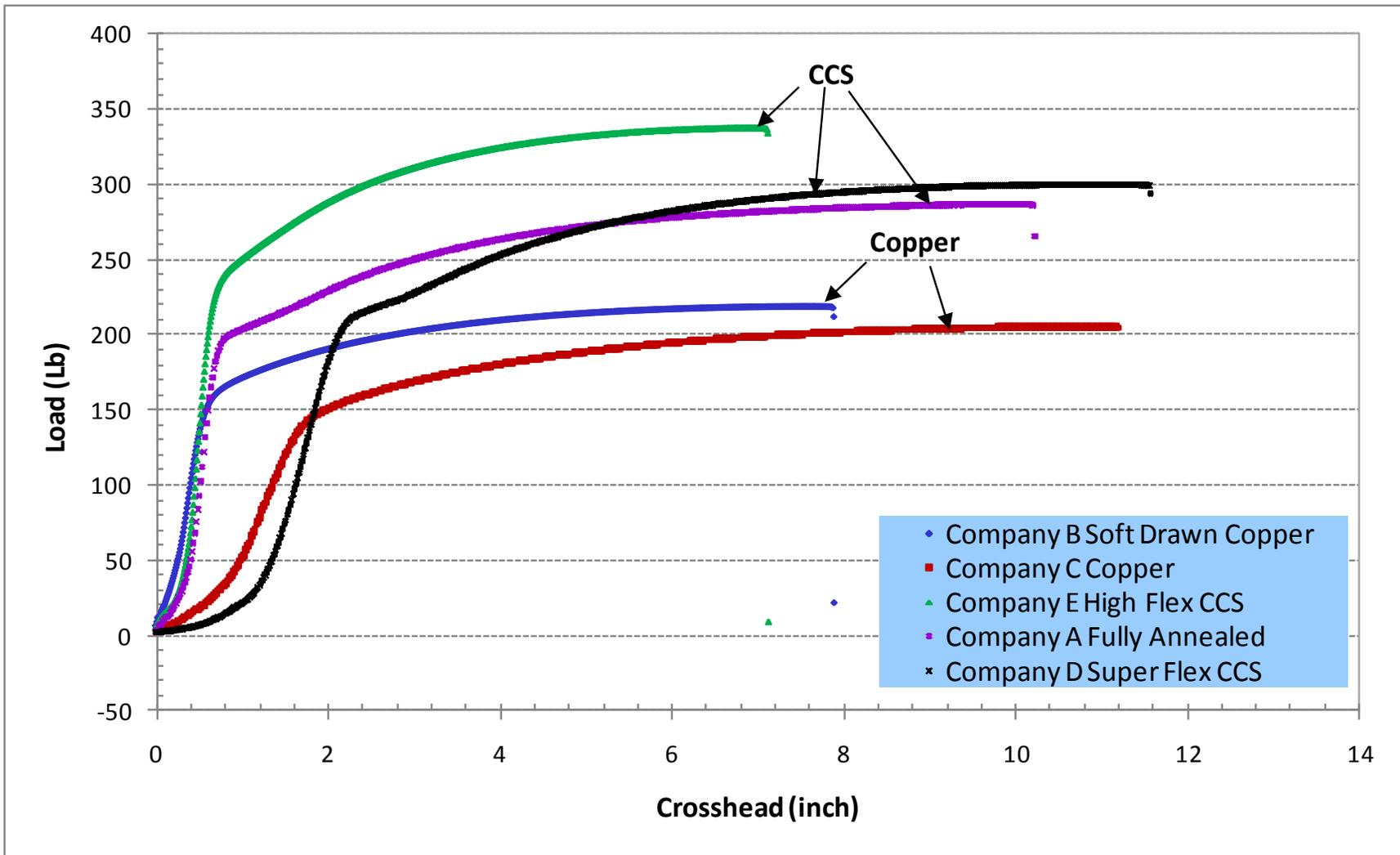
Figure 11. Tensile Plots of CCS vs. Soft Drawn Solid Copper Wires
