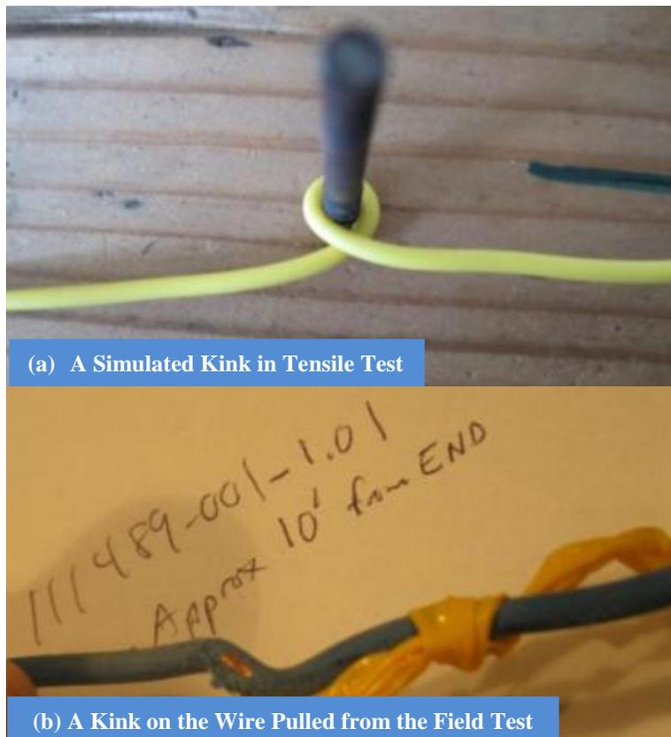
**Figure 1. The Simulated Kink for Tensile Test vs. a Kink on the Field Tested Wire**
