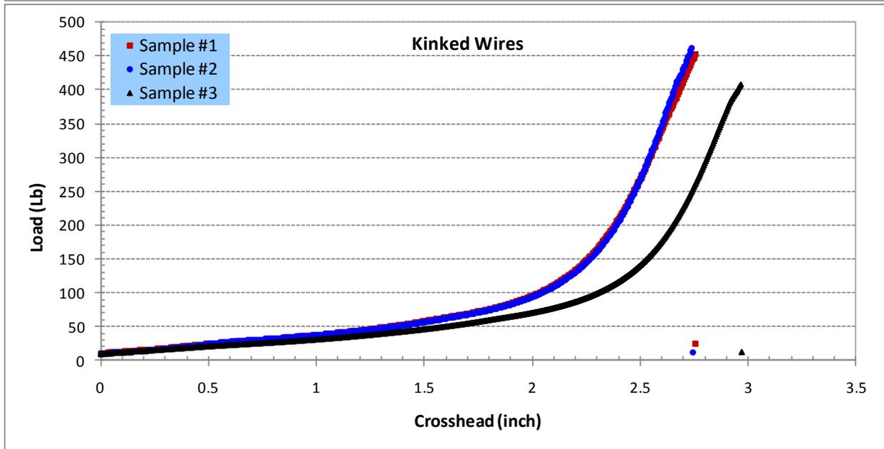
**Figure 30. Tensile Plots for Straight and Kinked Company D Extra High Strength 12 AWG Copper Clad Steel Wire**
