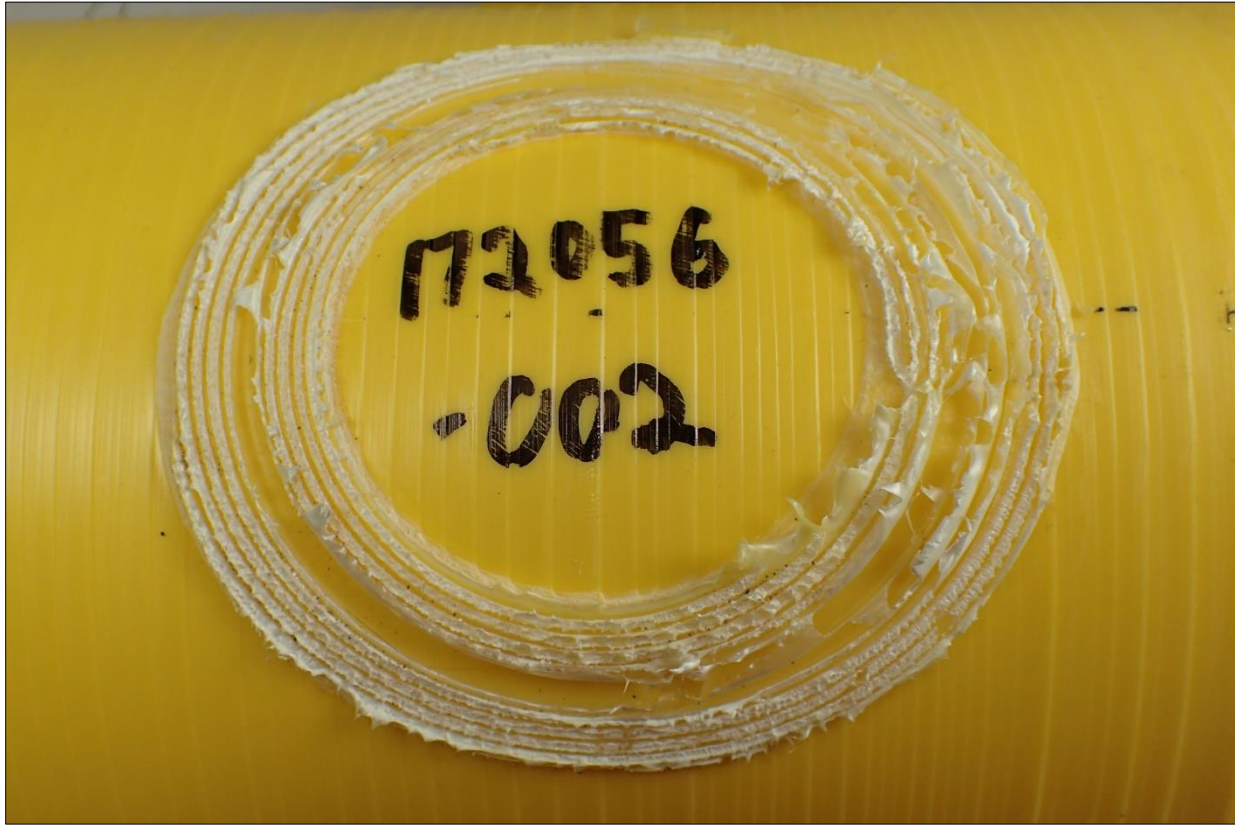
Figure 50. Decohesion test result, 4" IPS Frialen Peeler on MDPE pipe at -10°F
