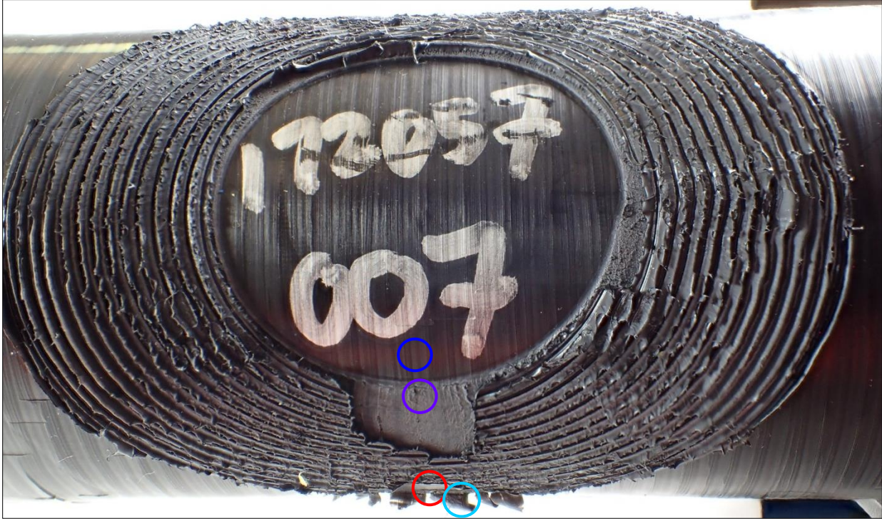
Figure 76. Decohesion test result, 2" IPS OEM Peeler on HDPE pipe at 120°F
