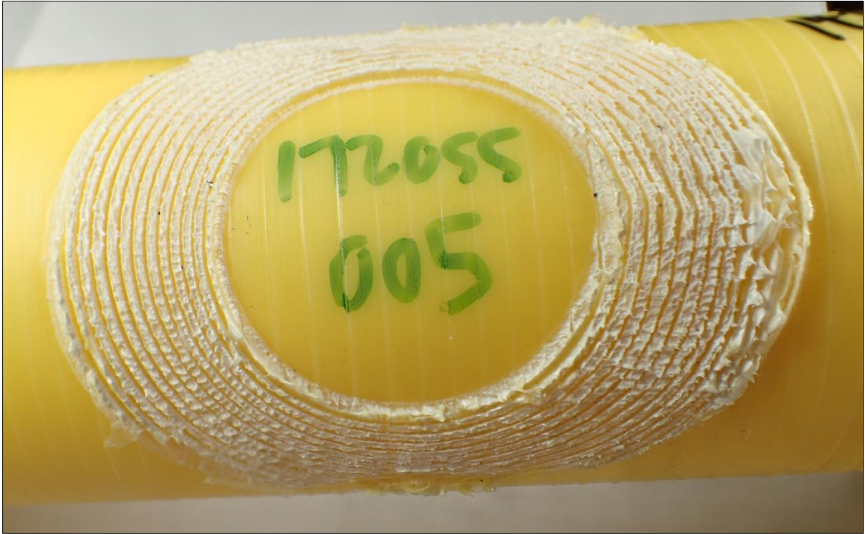
Figure 45. Decohesion test result, 2" IPS Frialen Peeler on MDPE pipe at 70°F
