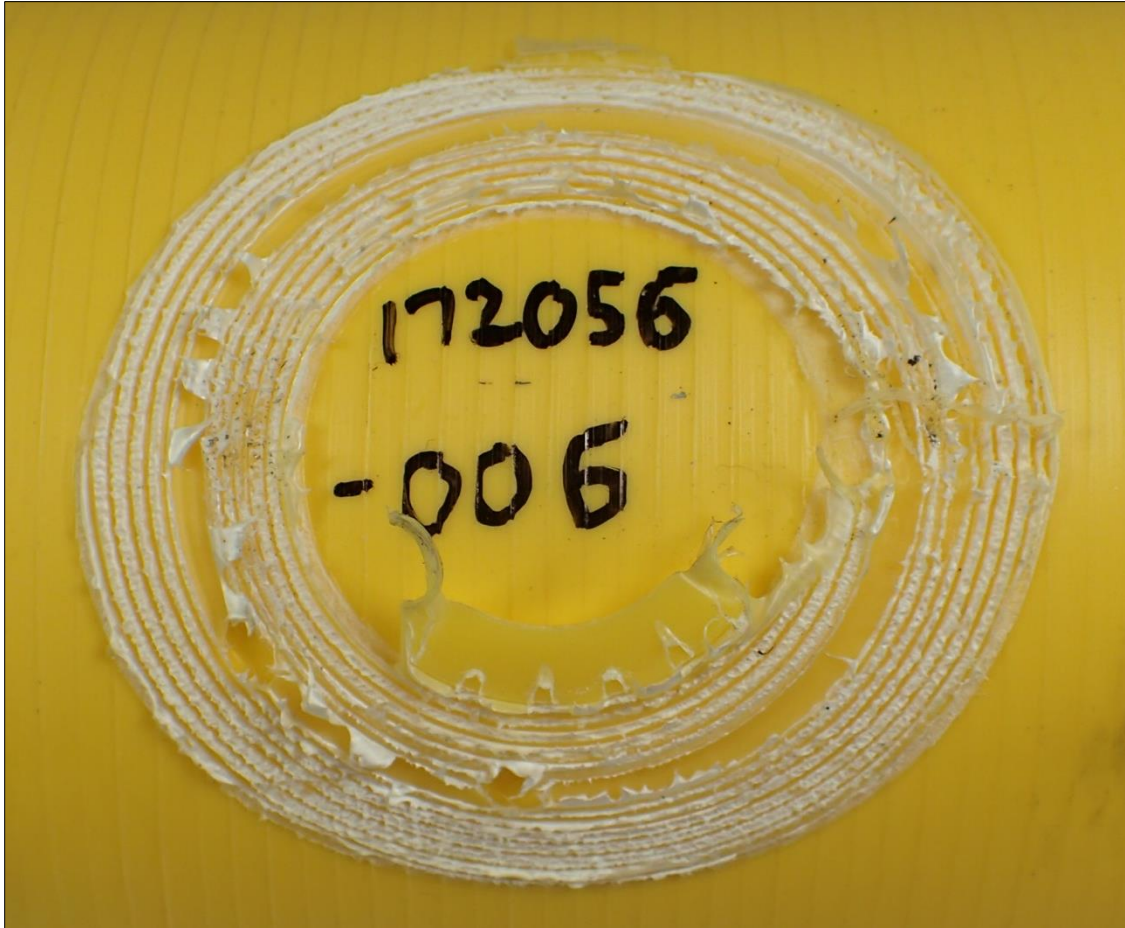
Figure 52. Decohesion test result, 4" IPS Frialen Peeler on MDPE pipe at 70°F
