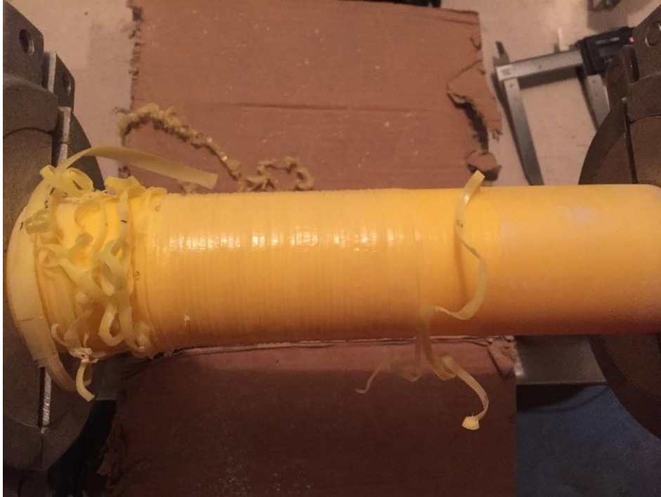
Figure 114: 2" IPS pipe with no induced ovality at 120°F, after scrape by OEM Scraper – with shavings around pipe
