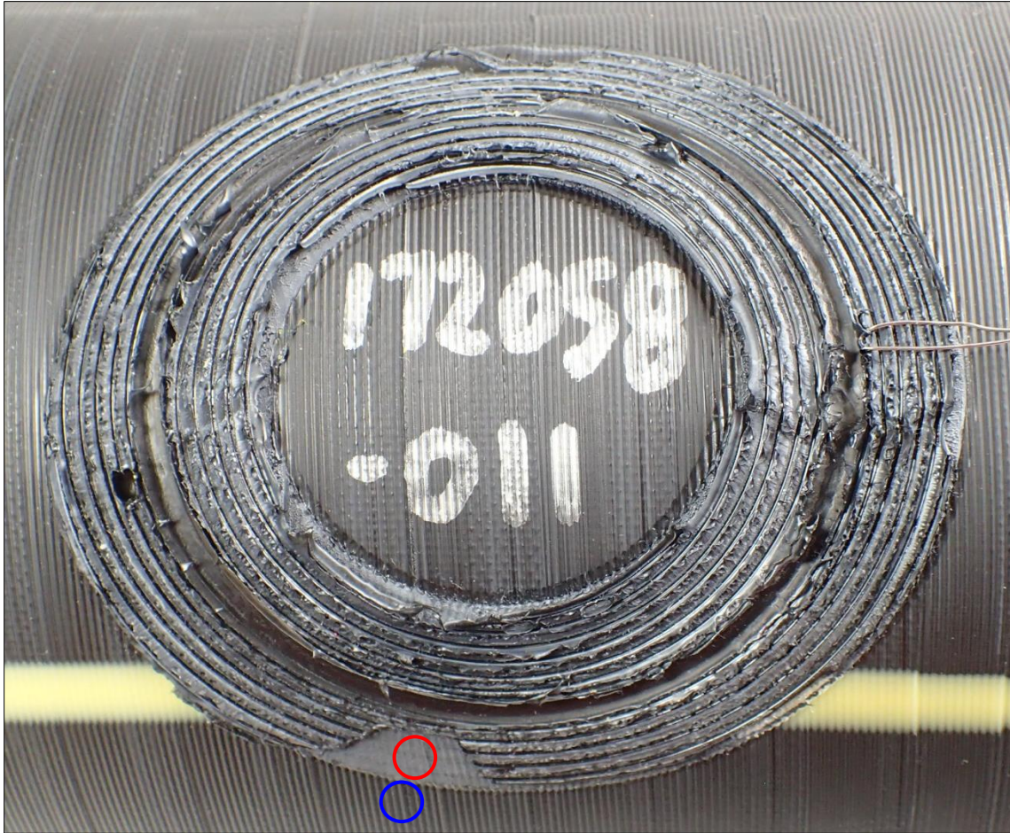
Figure 97. Decohesion test result, 4" IPS Summit rotary scraper on HDPE pipe at 120°F
