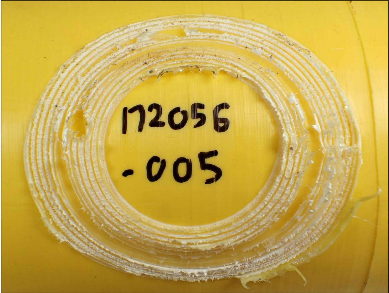
Figure 81. Decohesion test result, 4" IPS OEM Peeler on MDPE pipe at 70°F
