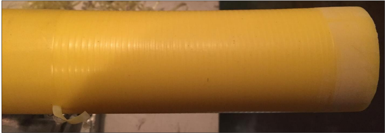
Figure 5. Typical scrape by 2" IPS Frialen Peeler
