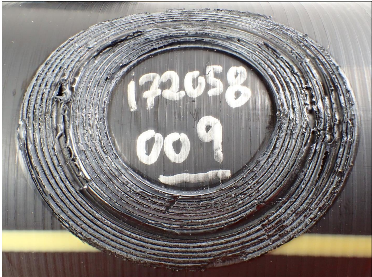
Figure 85. Decohesion test result, 4" IPS OEM Peeler on HDPE pipe at 120°F
