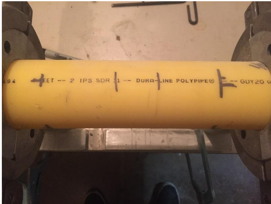
Figure 113: 2" IPS pipe with ~5% induced ovality at 70°F, before scrape – with bentonite powder contamination
