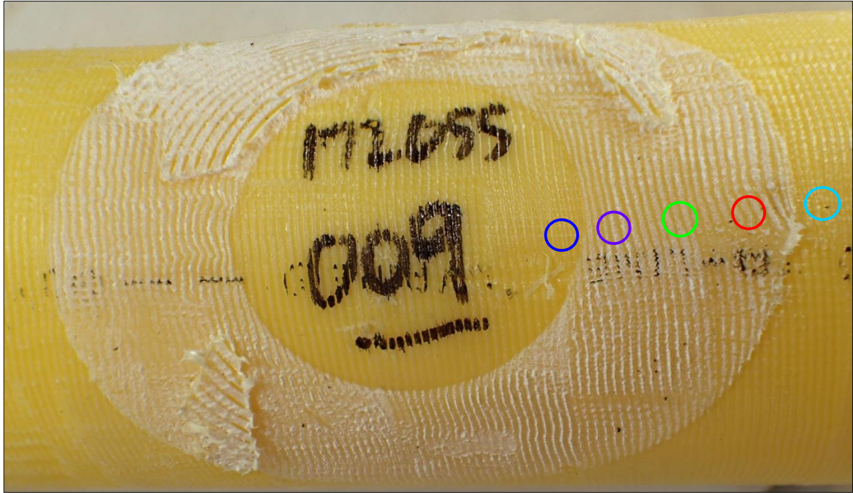
Figure 64. Decohesion test result, 2" IPS Half-Moon Scraper on MDPE pipe at 120°F
