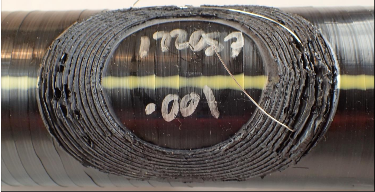
Figure 70. Decohesion test result, 2" IPS OEM Peeler on HDPE pipe at -10°F
