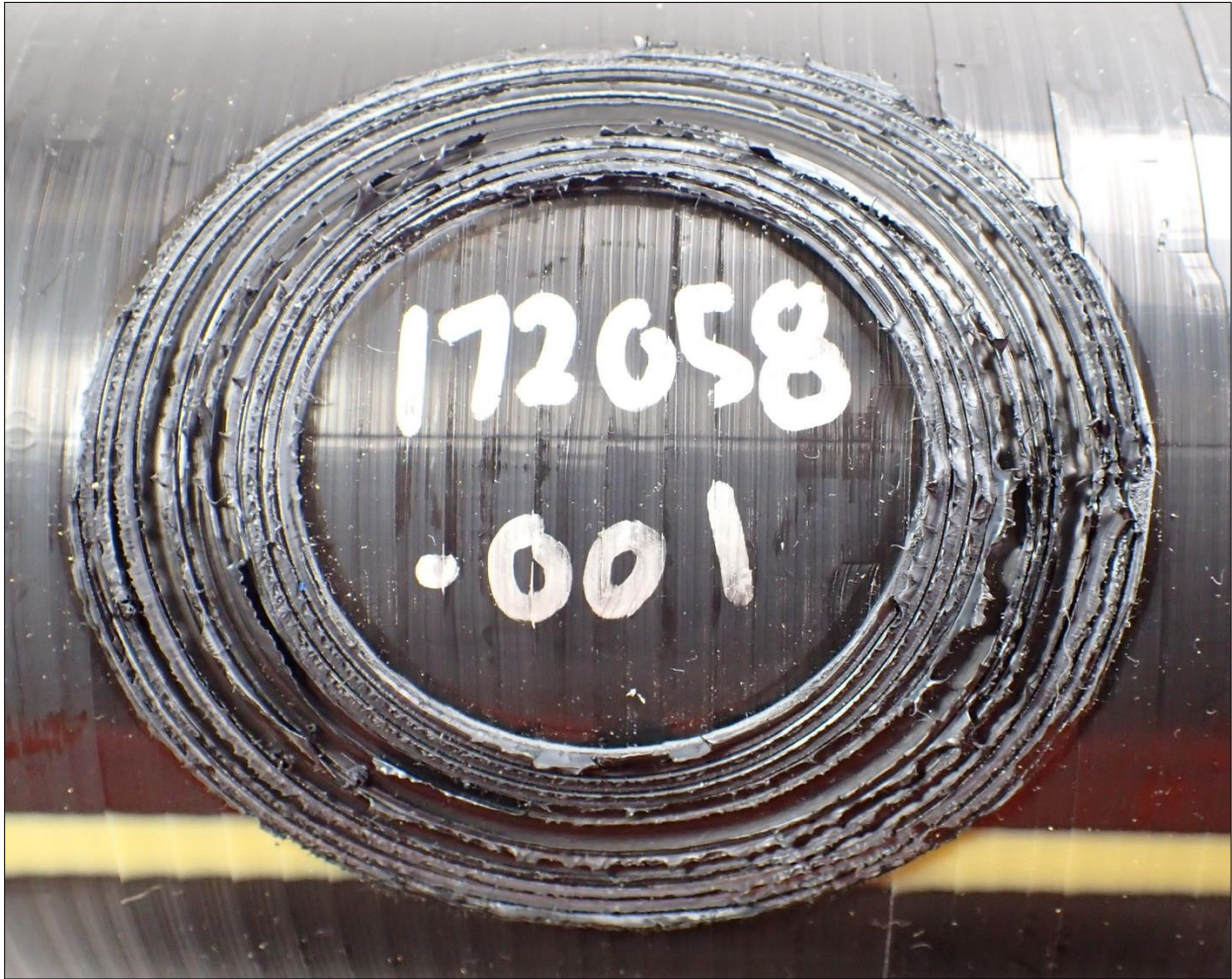
Figure 80. Decohesion test result, 4" IPS OEM Peeler on HDPE pipe at -10°F
