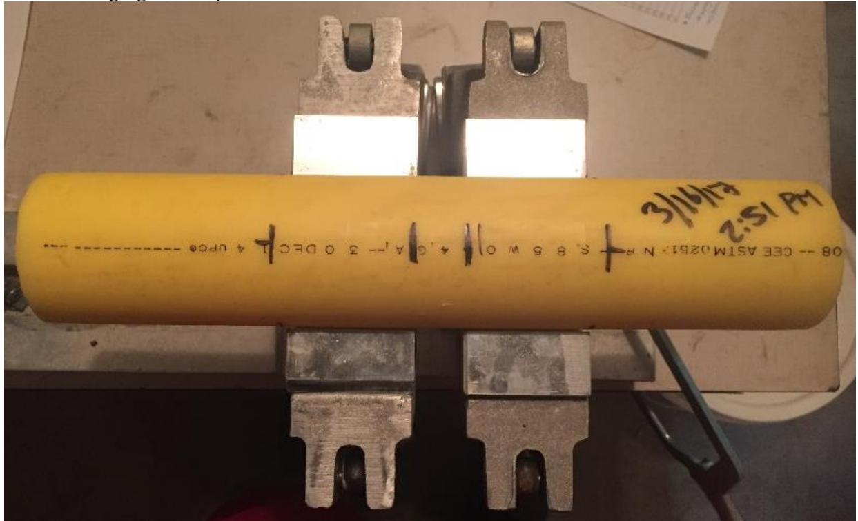
Figure 110: 2" IPS pipe clamps in pipe stands close together with pipe marked
