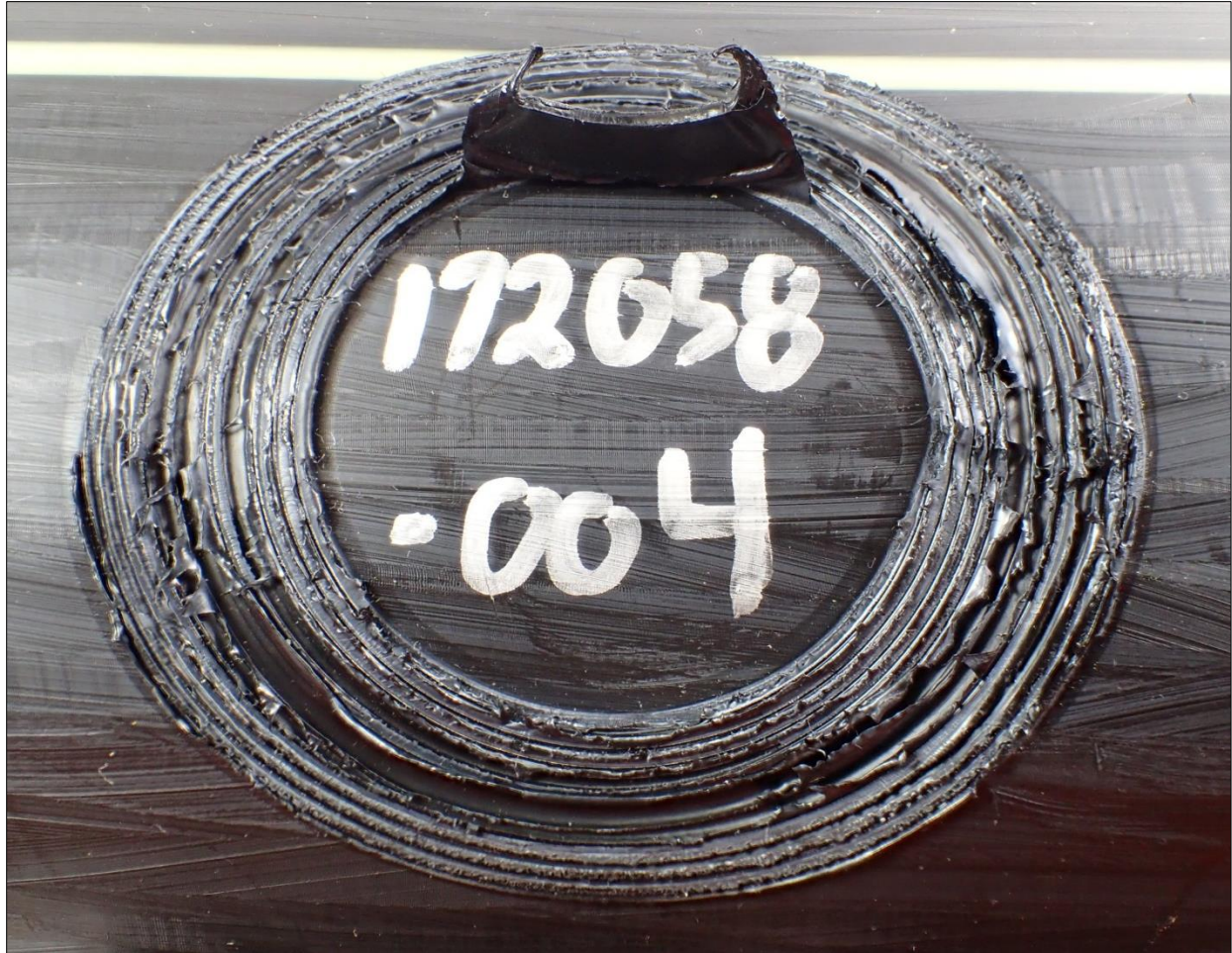
Figure 87. Decohesion test result, Friatec hand scraper on 4" IPS HDPE pipe at -10°F
