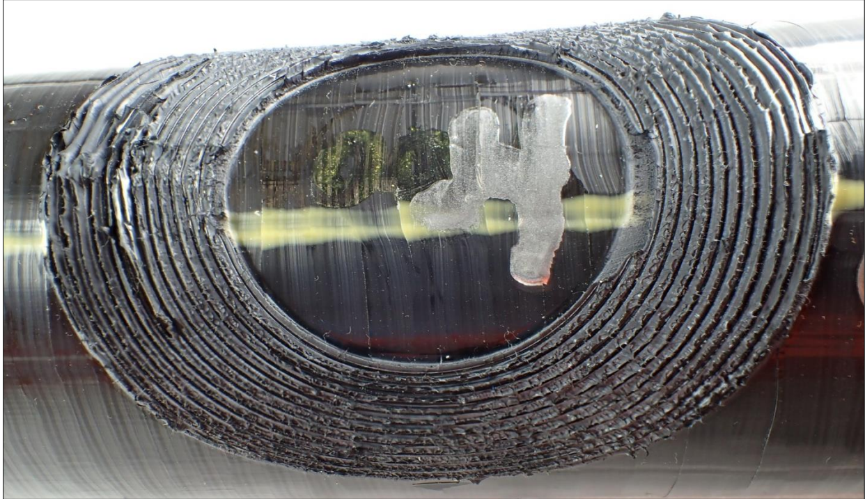
Figure 73. Decohesion test result, 2" IPS OEM Peeler on HDPE pipe at 70°F
