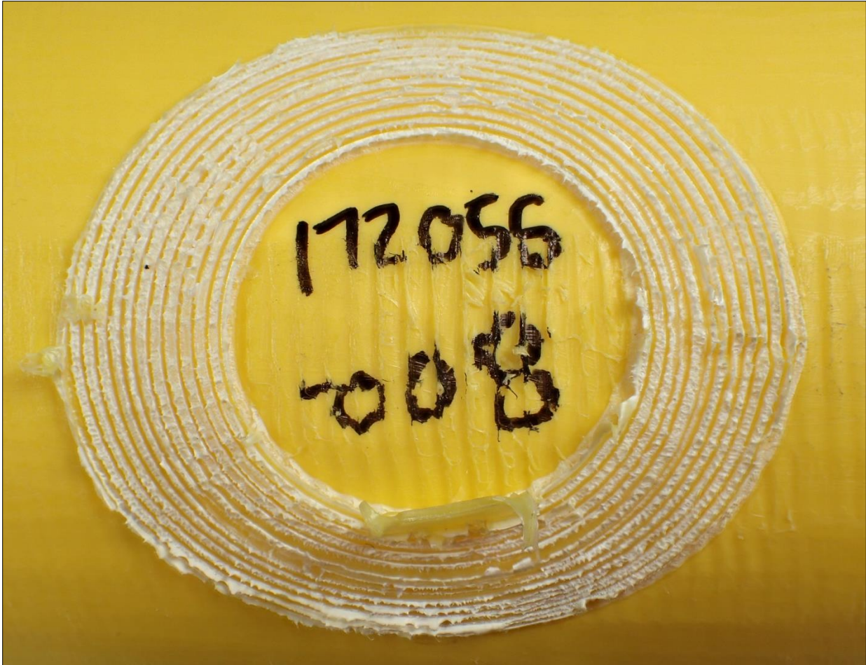
Figure 88. Decohesion test result, Friatec hand scraper on 4" IPS MDPE pipe at 70°F
