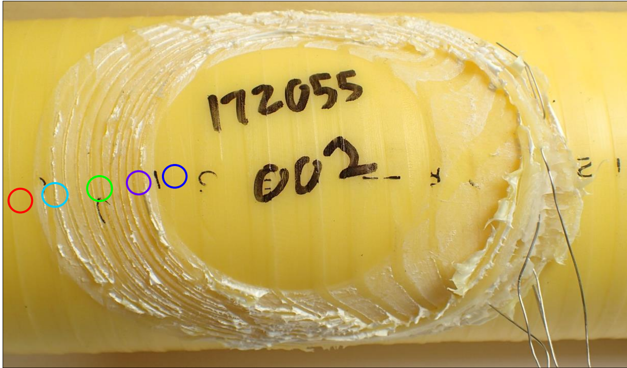
Figure 41. Decohesion test result, 2" IPS Frialen Peeler on MDPE pipe at -10°F
