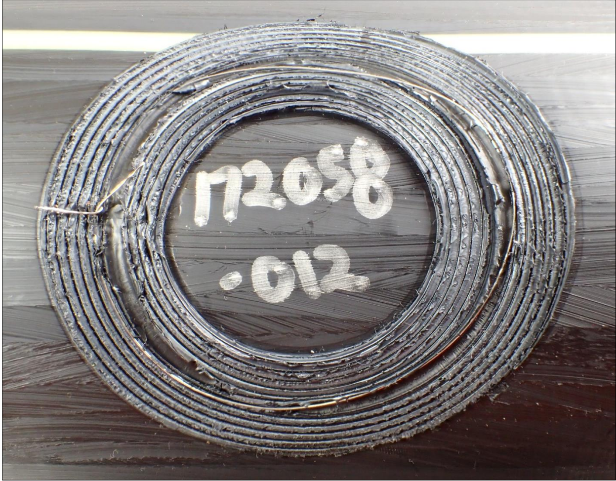
Figure 91. Decohesion test result, Friatec hand scraper on 4" IPS HDPE pipe at 120°F
