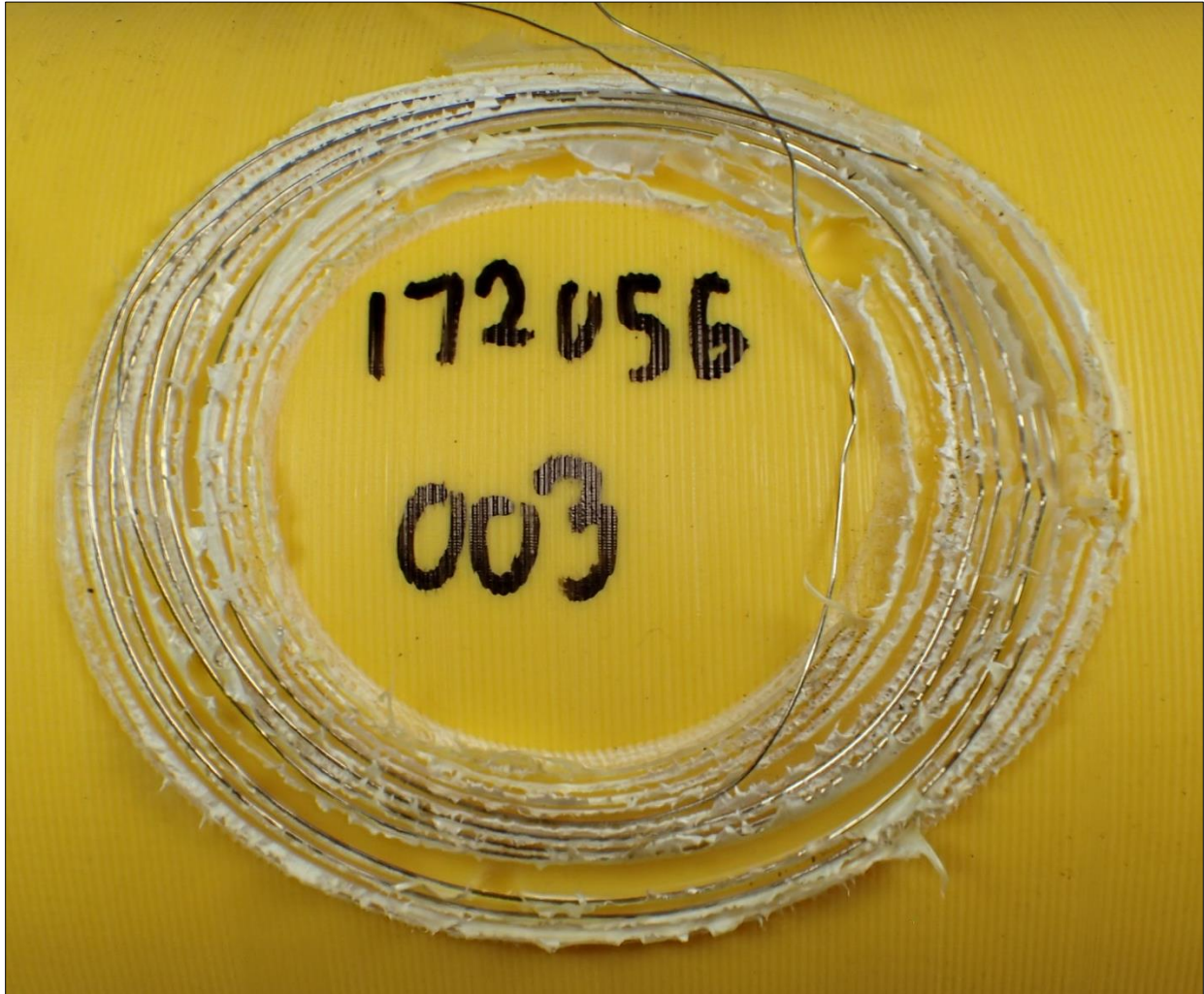
Figure 92. Decohesion test result, 4" IPS Summit rotary scraper on MDPE pipe at -10°F
