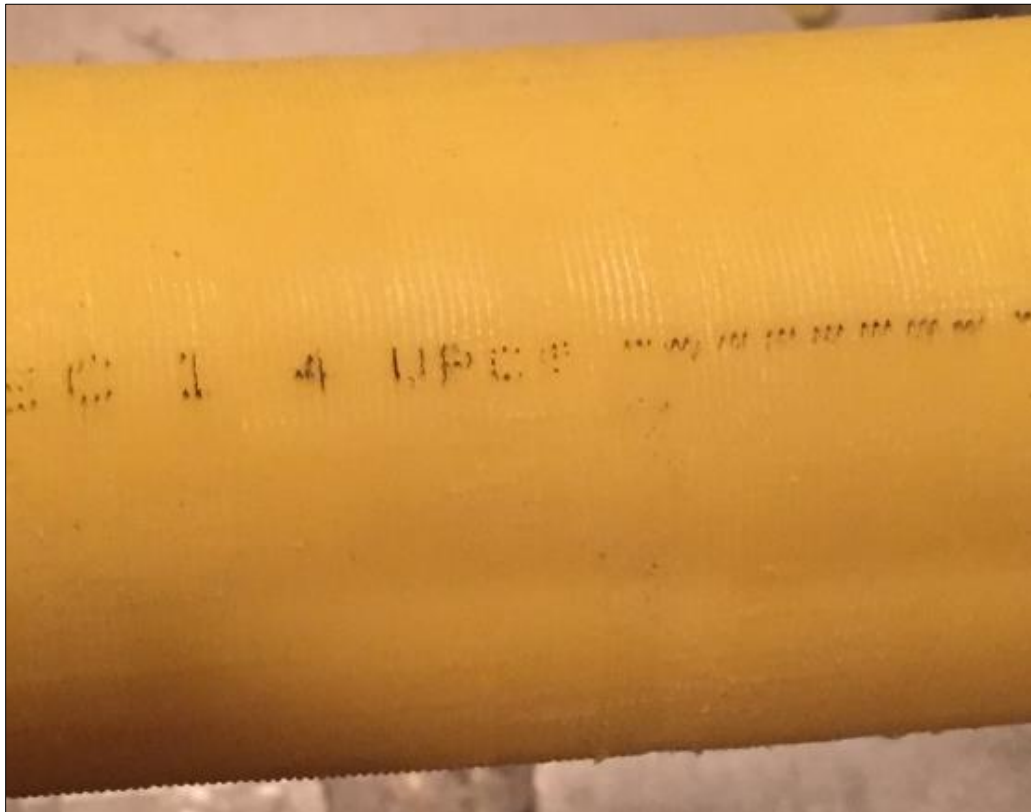
Figure 16. Typical scrape by 2" IPS Half-Moon Scraper (after several passes), closer view of serrated surface
