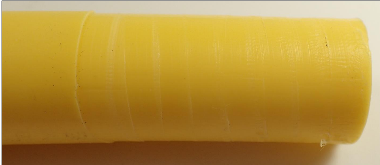
Figure 31. Typical scrape by ½" CTS Pencil Scraper
