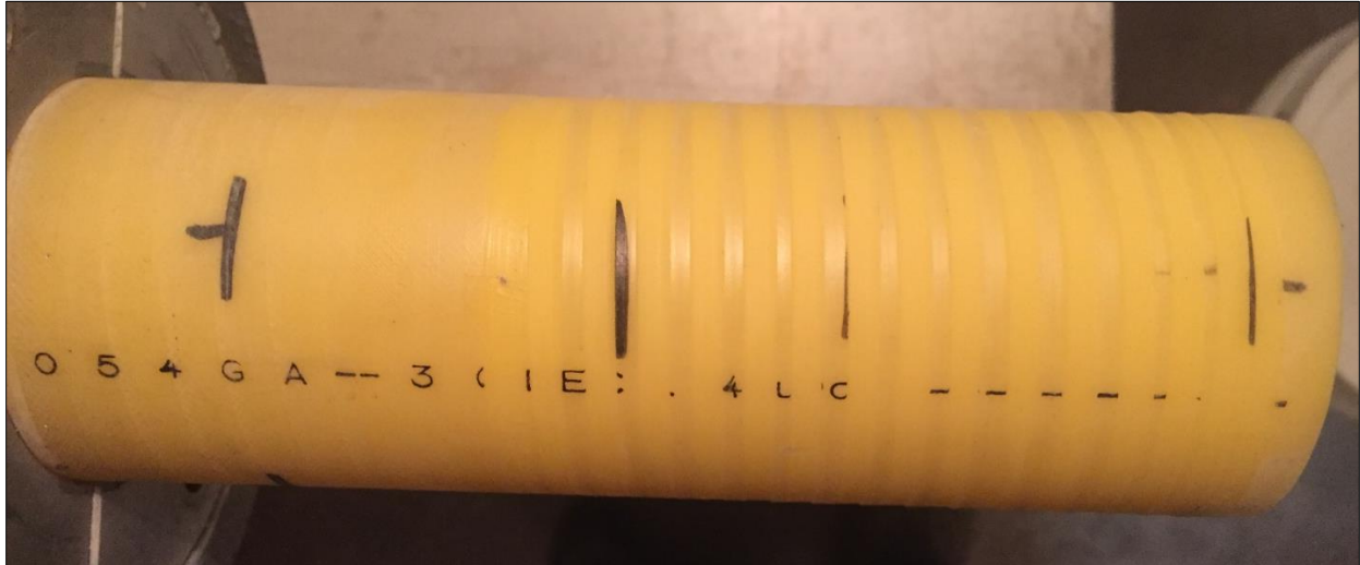
Figure 7. Non-scraped gaps left by 2" IPS Frialen Peeler
