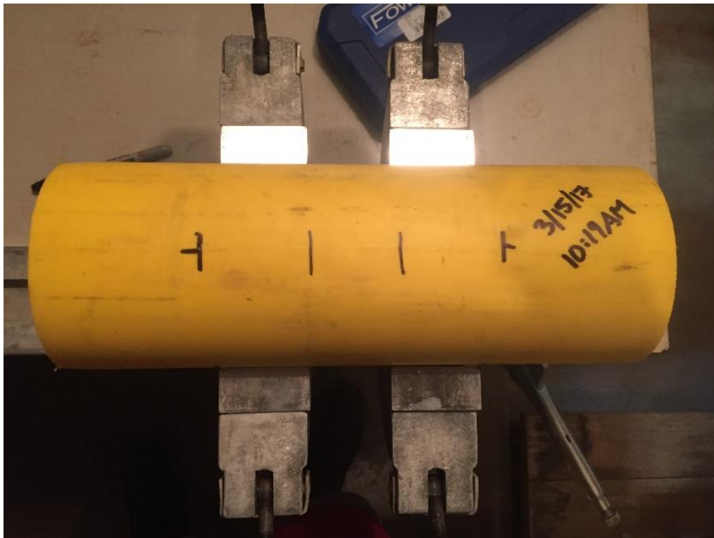
Figure 111: 4" IPS pipe clamps in pipe stands close together with pipe marked
