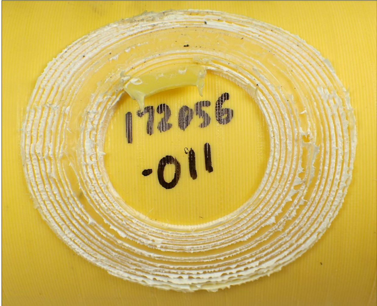
Figure 96. Decohesion test result, 4" IPS Summit rotary scraper on MDPE pipe at 120°F
