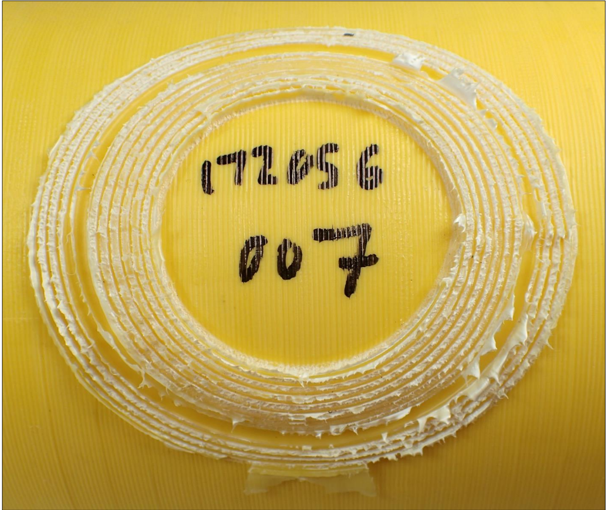
Figure 94. Decohesion test result, 4" IPS Summit rotary scraper on MDPE pipe at 70°F
