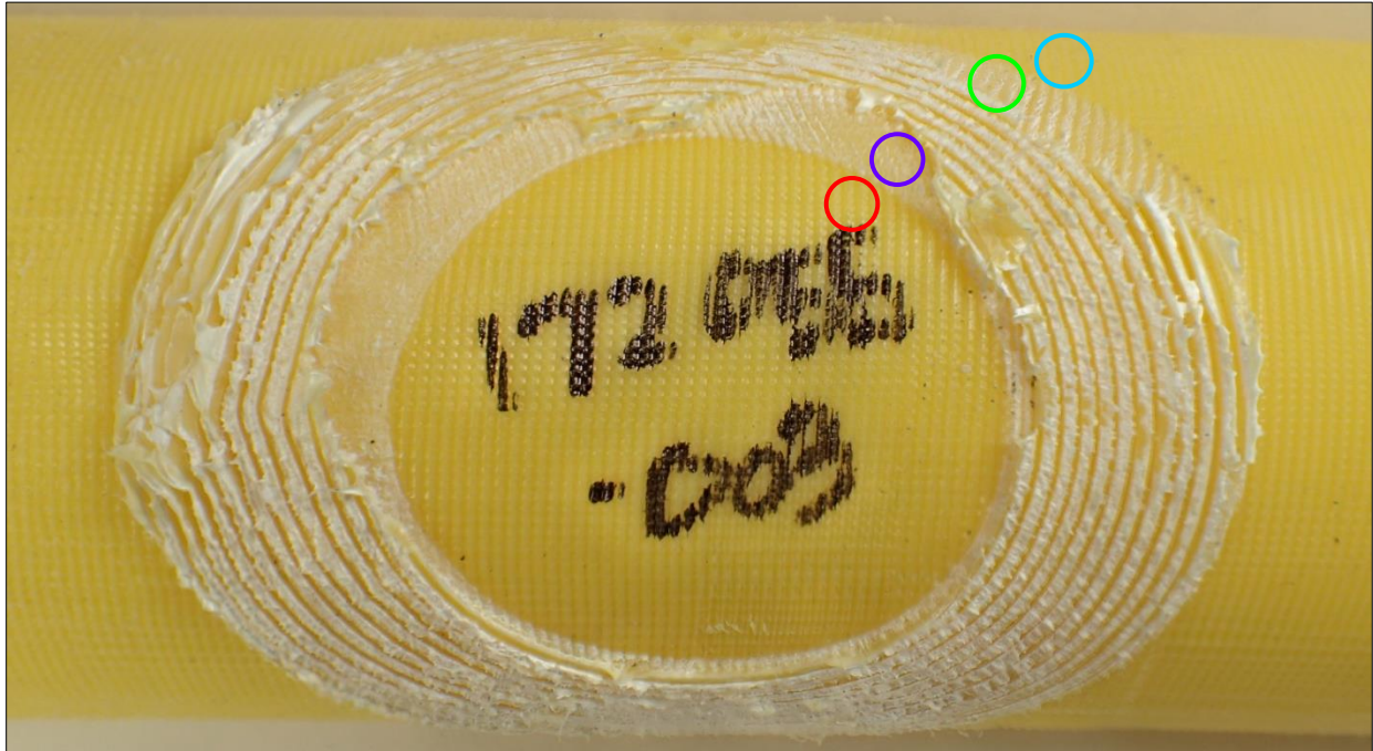
Figure 58. Decoherion test result, 2" IPS Half-Moon Scraper on MDPE pipe at -10°F
