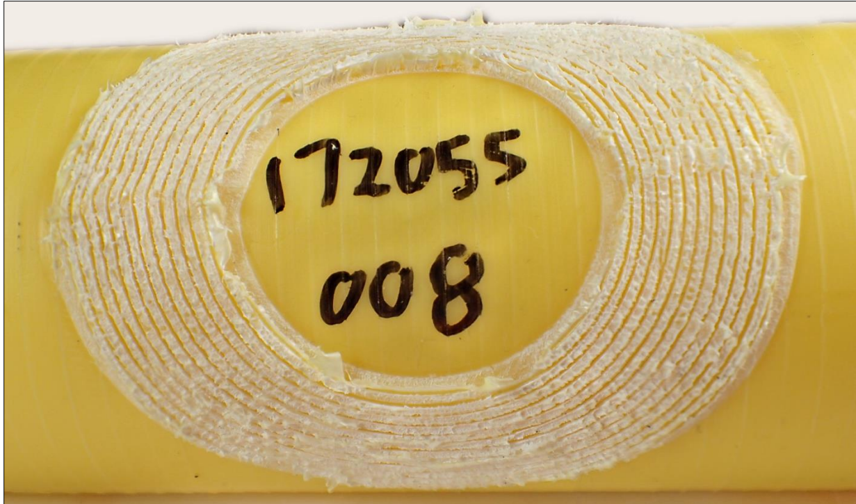
Figure 48. Decohesion test result, 2" IPS Frialen Peeler on MDPE pipe at 120°F
