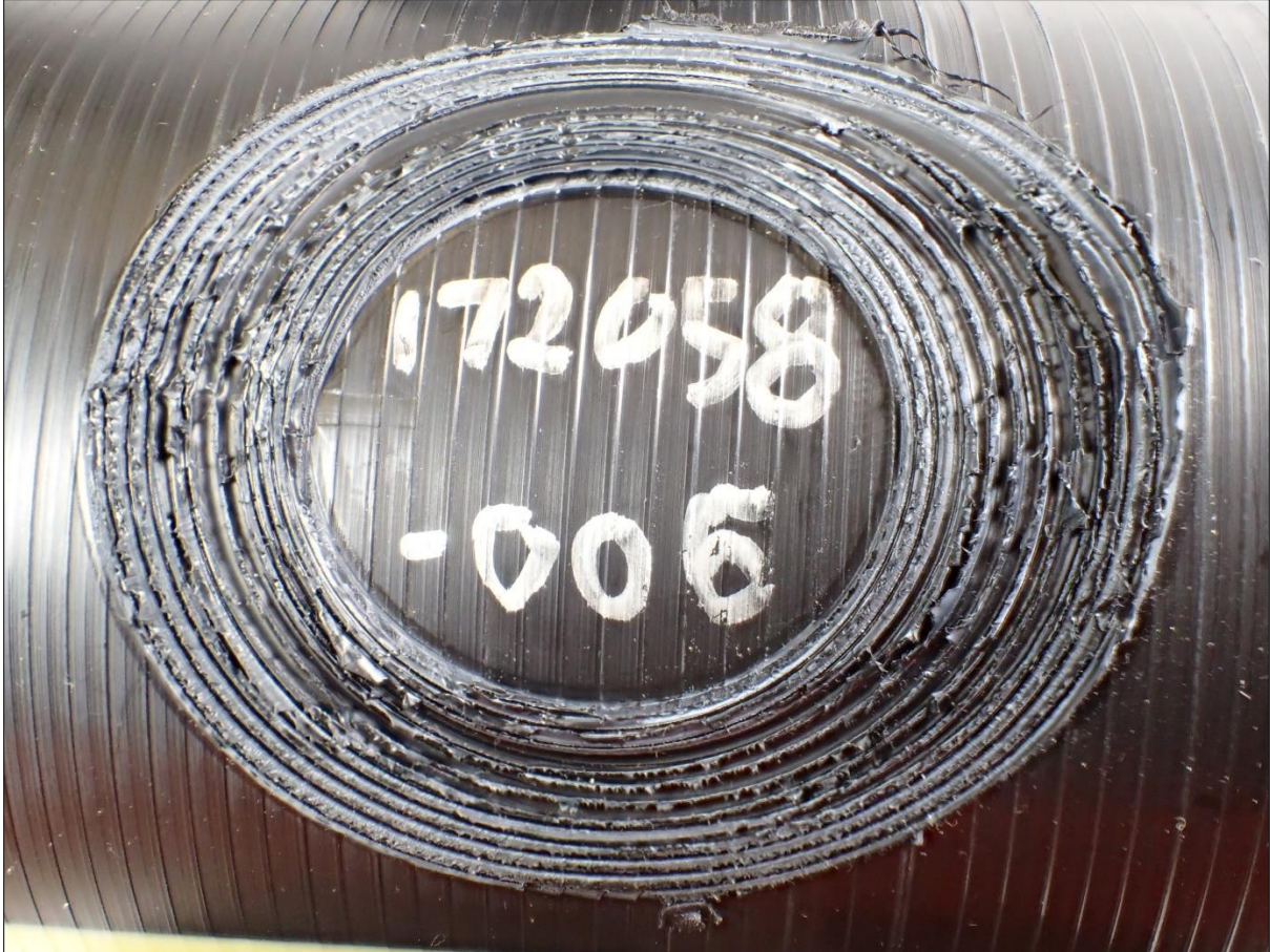
Figure 53. Decohesion test result, 4" IPS Frialen Peeler on HDPE pipe at 70°F
