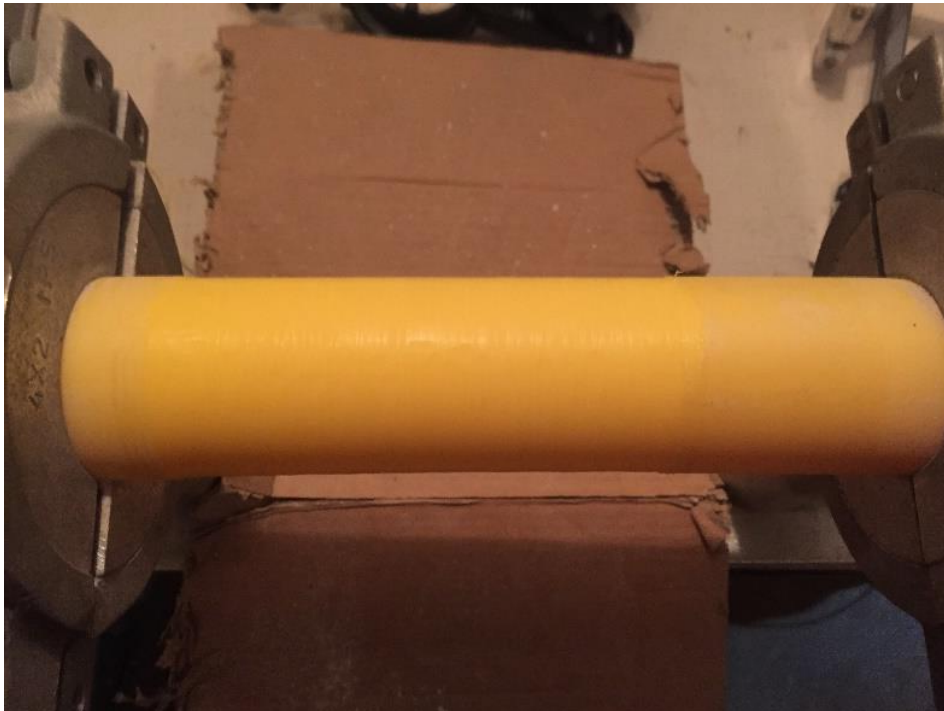
Figure 115: 2" IPS pipe with no induced ovality at 120°F, after scrape by OEM Scraper – after removal of shavings
