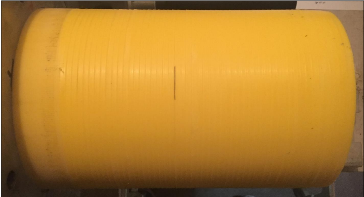
Figure 11. Typical scrape by 4" IPS Frialen Peeler
