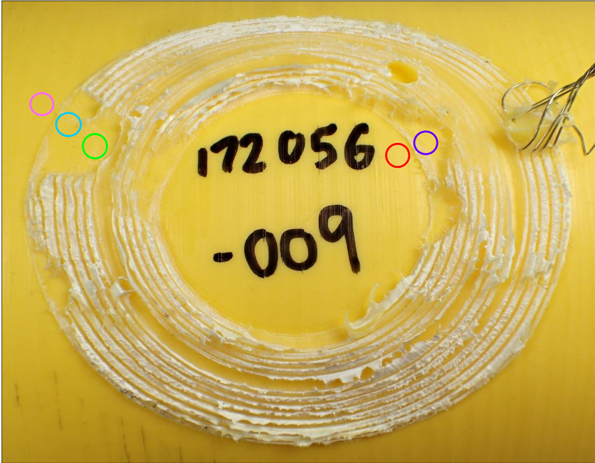
Figure 83. Decohesion test result, 4" IPS OEM Peeler on MDPE pipe at 120°F
