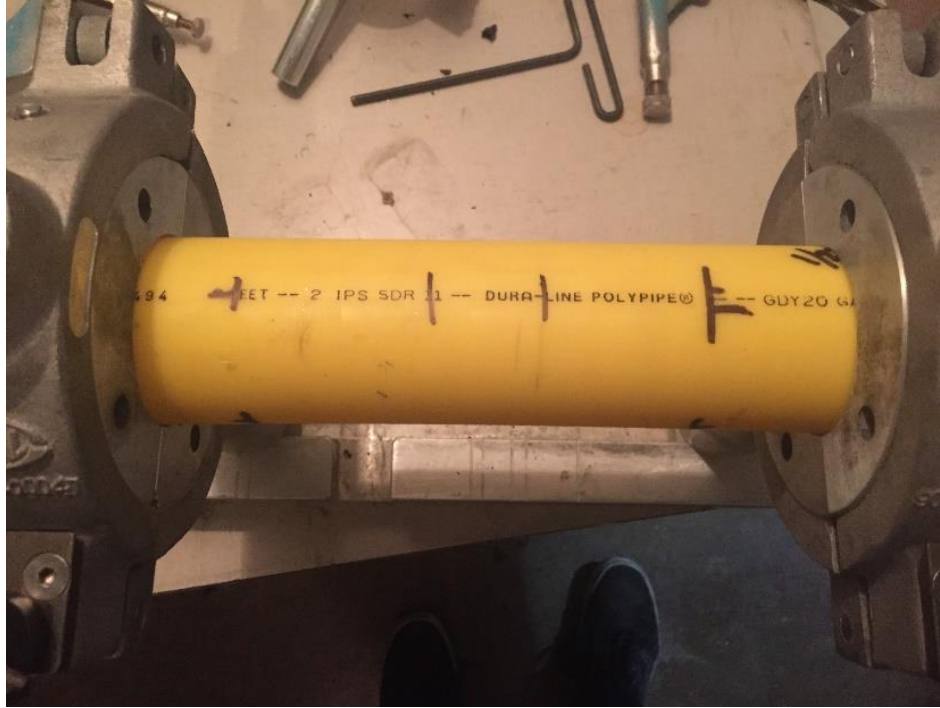
Figure 112: 2" IPS pipe with ~5% induced ovality at 70°F, before scrape – no contamination
