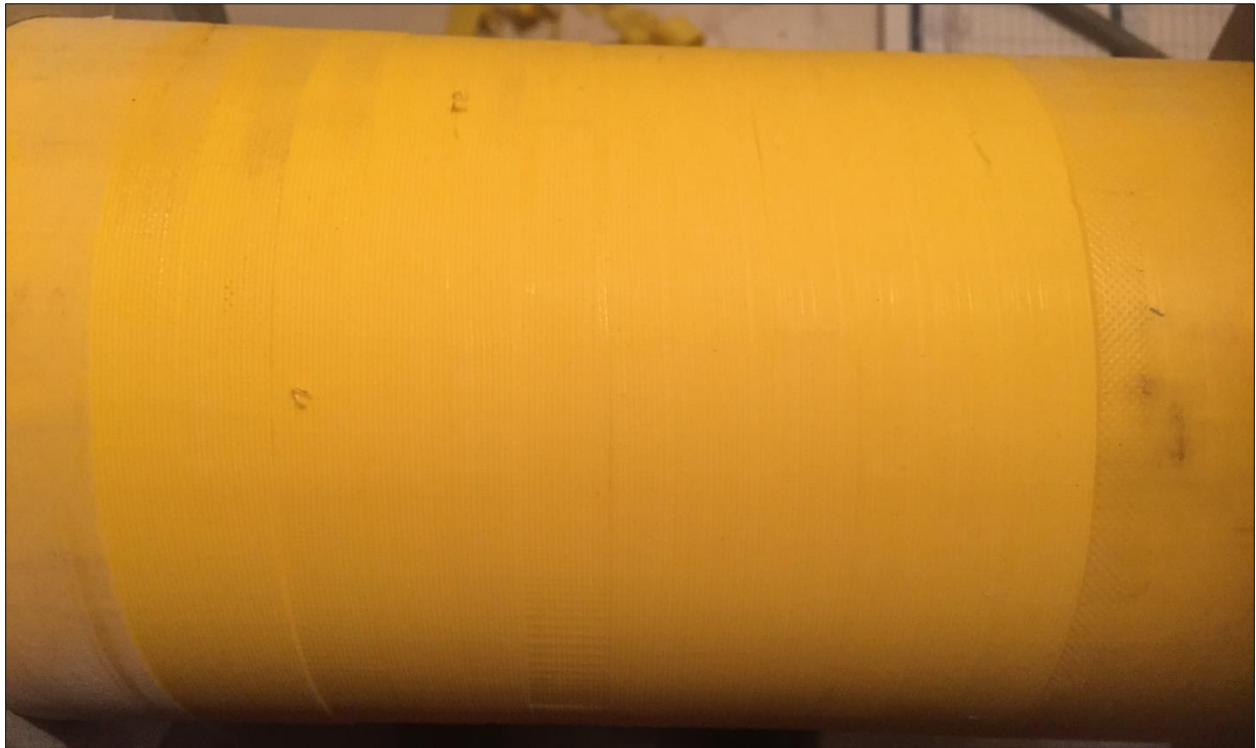
Figure 35. Typical scrape by 4" IPS Summit Rotary Scraper
