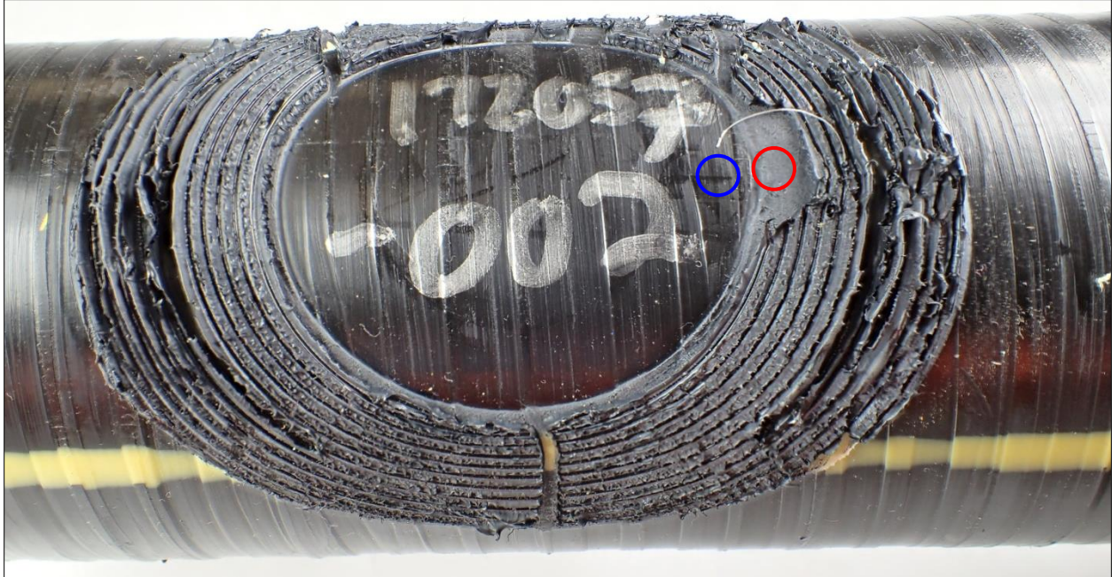
Figure 43. Decohesion test result, 2" IPS Frialen Peeler on HDPE pipe at -10°F
