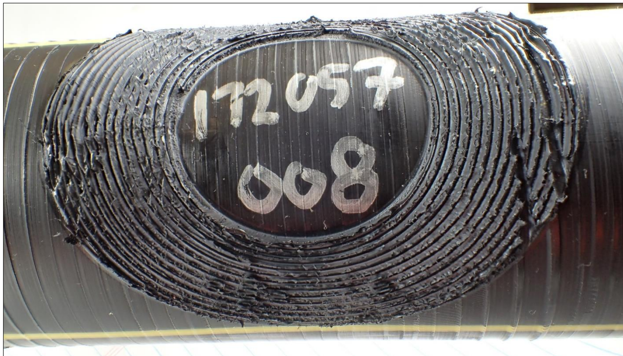
Figure 49. Decohesion test result, 2" IPS Frialen Peeler on HDPE pipe at 120°F
