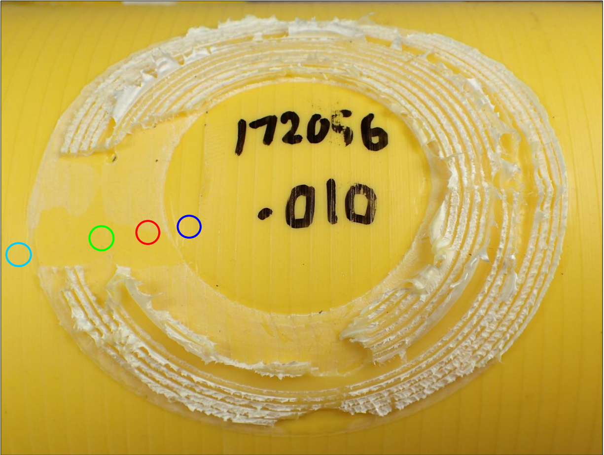
Figure 54. Decohesion test result, 4" IPS Frialen Peeler on MDPE pipe at 120°F
