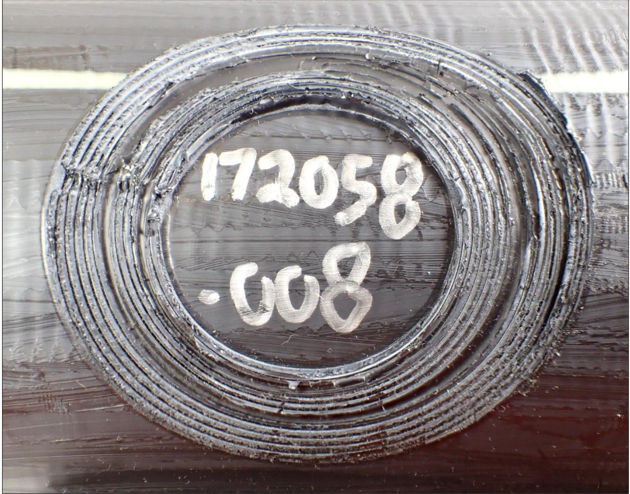
Figure 89. Decohesion test result, Friatec hand scraper on 4" IPS HDPE pipe at 70°F
