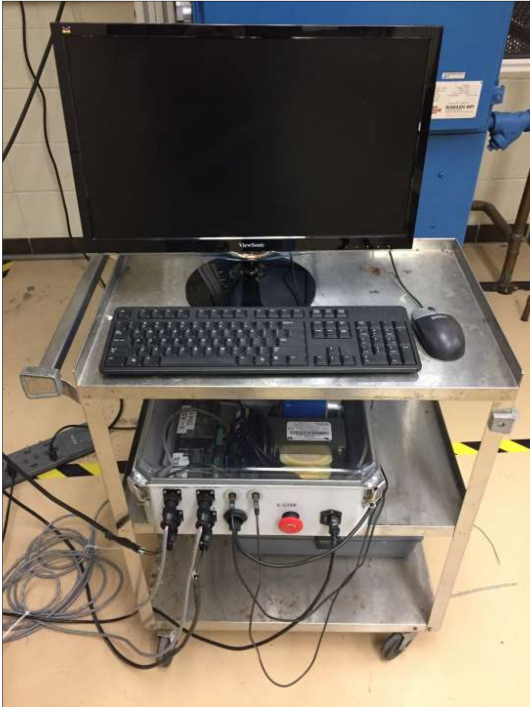
Figure 30. Pipe contaminator control console and electronics box
