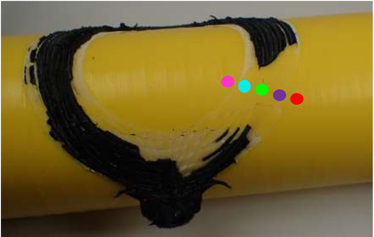
Figure 109. Sample 172318-042, decohesion test result
