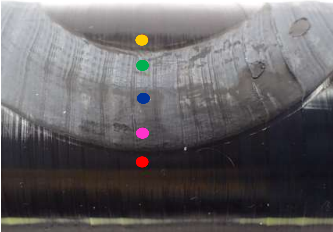
Figure 217. Sample 172316-075, decohesion test result
