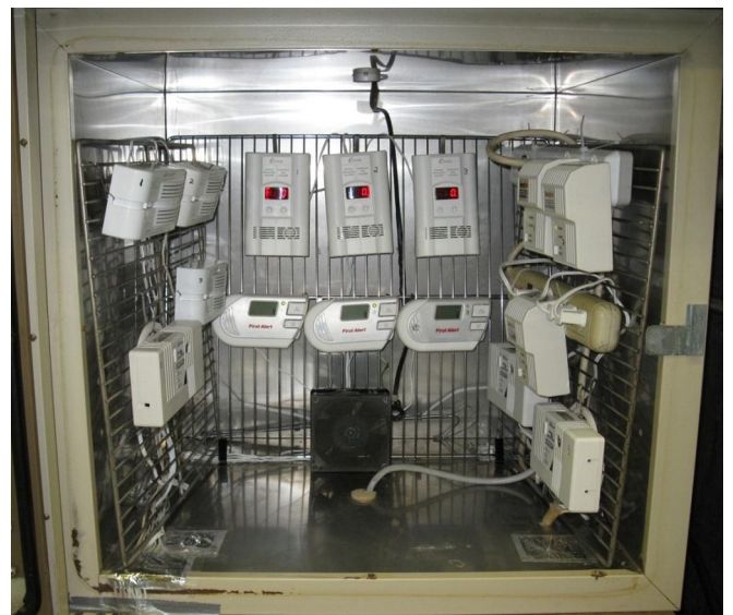
Detectors were tested in a specially designed test chamber at Gas Technology Institute facilities.
